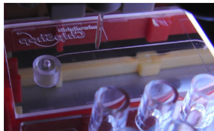
Fig. 746: instrument TWO-300P spotting in microfluidic devices DNA-Array embedded in a microfluidic channel
