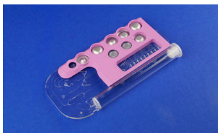
Fig. 1010: Real-time PCR chip for B-agent detection, Horizon 2020 project, No. 700264
