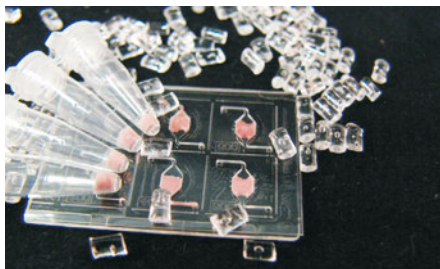
Fig. 960: PCR chip with integrated freeze-dried master mix
