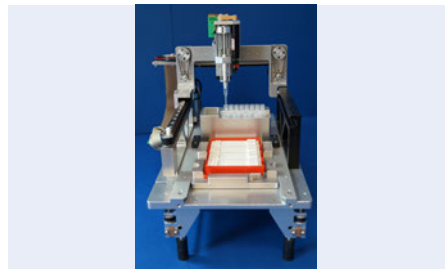
Fig. 987: Merger of standard liquid handling and lab-on-a-chip technology – LOC pipettor & xy-stage for optical read out, TAB project No. 2011 FE 9023
