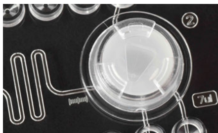
Fig. 446: Rotary valve with triangular recess for valve actuator
