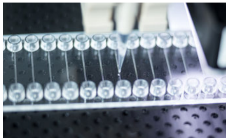
Fig. 744: instrumentTWO-300P spotting in microfluidic devices DNA-Array embedded in a microfluidic channel
