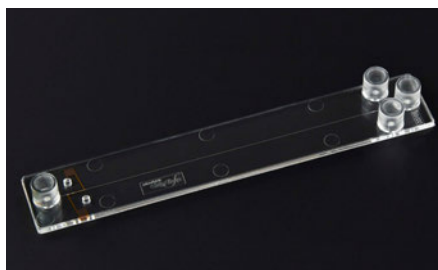
Fig. 75: Cross-shaped channel chip with electrodes for contactless conductivity detection
