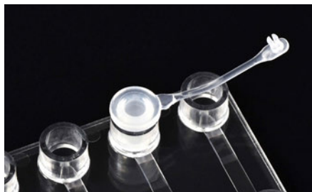
Fig. 606: Male Luer plug Fluidic 264 with retaining stripe on chip
