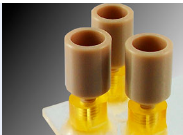
Fig. 633: Cross-shaped channel chip with three bonded port connectors and three chip reservoirs
