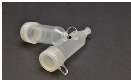
Fig. 679: Sampling vessel with pierceable septum
