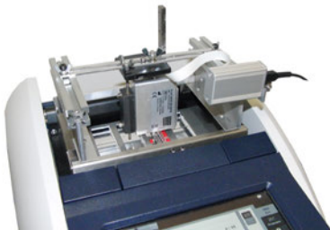
Fig. 832: Implementation of low-volume real-time PCR on chip – Chip on breadboard instrument
