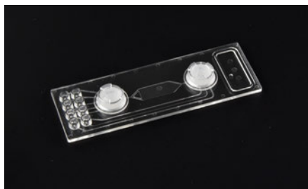
Fig. 536: Assay chip 3 – Fluidic 490 with central reaction chamber and integrated turning valve for fluid actuation
