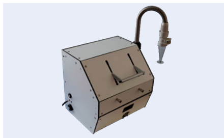
Fig. 992: Breadboard system: Electrochemical immunoassay system for air sample analysis, FP7 project Multisense Chip, No. 261810
