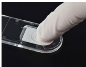
Fig. 944: Sample uptake via active finger pump
