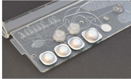
Fig. 639: Blister pouches of different volumes integrated in a complex microfluidic chip
