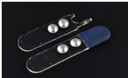
Fig. 947: Unstructured handheld platform for prototyping with sample uptake interface
