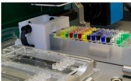
Fig. 227: 65-well chip used as source plate in spotter
