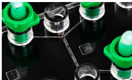
Fig. 183: One unit of the Herringbone mixer chip Fluidic 187, equipped with Luer to fluid connectors and tubing
