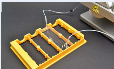
Fig. 869: Chip with olives connected via tubes to a peristaltic pump
