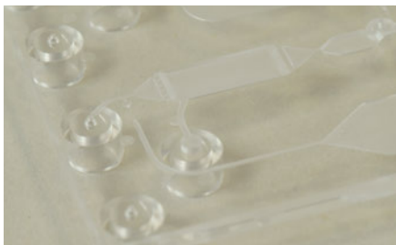
Fig. 895: Details of channels and chambers produced by milling a thermoplastic polymer platform
