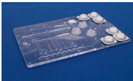
Fig. 1002: Integrated microfluidic chip for the detection of bacterial pathogens, FP7 project Multisense Chip, No. 261810
