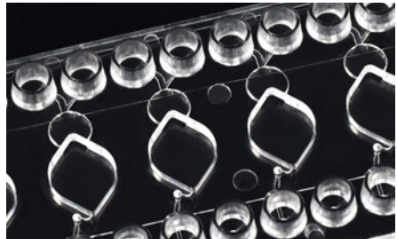
Fig. 209: Snowman head, to be preloaded with 5 µl sample, subsequent addition of 45 µl diluent enables efficient mixing in snowman belly
