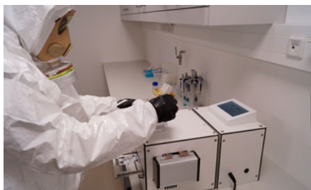
Fig. 1003: Multisense Chip Analyzer: Demonstration of detection of airborne bacterial pathogens, FP7 project Multisense Chip, No. 261810
