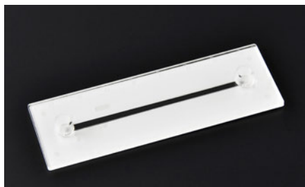
Fig. 468: Straight channel chip Fluidic 268 with double-sided adhesive tape
