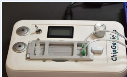
Fig 881: Chip inserted into ChipGenie® edition P instrument and installed connectors with silicone sleeve and PTFE tubing.
