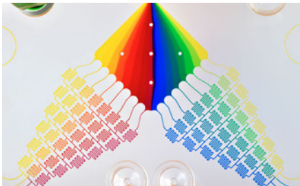
Fig. 435: The 2D Gradient Generator chip can be used to generate various gradients, e.g. of drug concentrations or color
