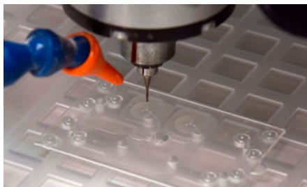
Fig. 894: Milling of various design features using a standardized interface platform
