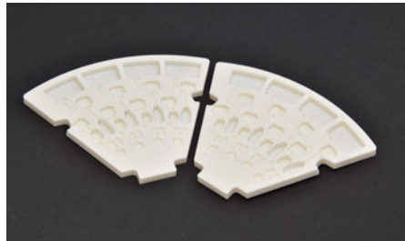
Fig. 938: Examples of pie slice plate chips. The chips were developed within the BMBF-Project "Zentrilab", FKZ 16SV2350.
