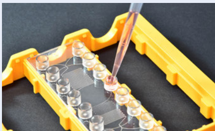
Fig. 856: Microfluidic chip with Luer interfaces filled with a pipette and interfaces used as reservoir
