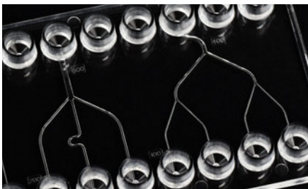
Fig. 170: Detail of the splitter units dividing one stream into three or four streams with varying channel sizes
