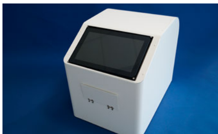
Fig. 1005: Analyzer for molecular detection of viral pathogens in the food supply chain, FP7 project EDEN, No. 313077
