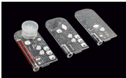
Fig. 951: Cartridges for the detection of tuberculosis, early HIV infection, and liver function (from left to right)
