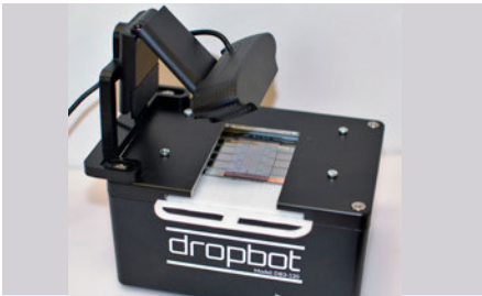
Fig. 741: DropBot instrument for manipulation and read-out
