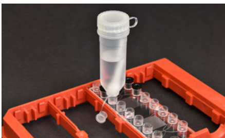
Fig. 678: Sampling vessel prefilled with buffer and inserted swab
