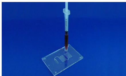
Fig. 980: Boyle-Marriott PCR chip for ultrafast PCR, design: IMM, realized within the FP 7 project "CD-Medics", No. 216031
