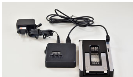
Fig. 736: Complete setup of the Lab-on-a-Chip Cell Culture Incubator – LOC CCI 1 with temperature control unit
