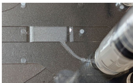
Fig. 548: Introduction of Agarose beads into the trapping chamber of chip Fluidic 1530
