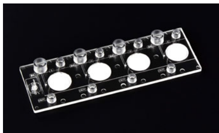
Fig. 304: Plasma/serum generation chip Fluidic 168 equipped with plasma generation membranes
