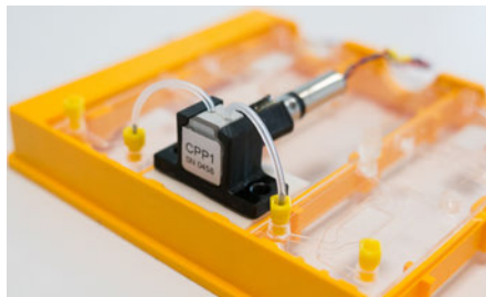
Fig. 794: CPP1 pump mounted on a handling frame via a holder (black) and connected to chips in slide format
