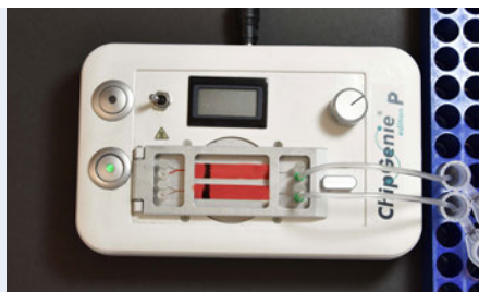
Fig 882: ChipGenie® edition P instrument with a blood sample inside the rhombic chamber. The magnetic beads, migrating through the chambers, are visible as black bars.
