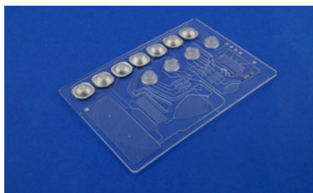
Fig. 996: Integrated microfluidic chip with complete sample preparation for miRNA analysis, BMBF project IMRA, FKZ 0316078A
