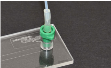
Fig. 12: A Luer connector mounted on a Luer interface with attached tubing
