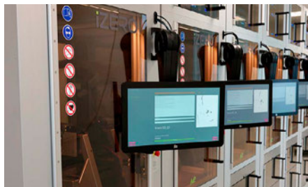
Fig. 899: Spotter technology available at microfluidic ChipShop for reagent integration
