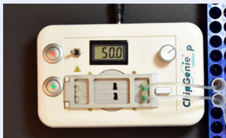
Fig. 883: ChipGenie® edition P instrument with washing buffer inside the rhombic chamber.
