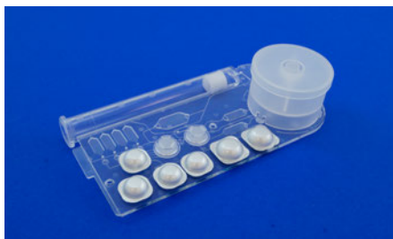
Fig. 1009: Immunoassay-Chip for mycotoxine analysis, BMBF-Project Kombispec, FKZ 13N13757
