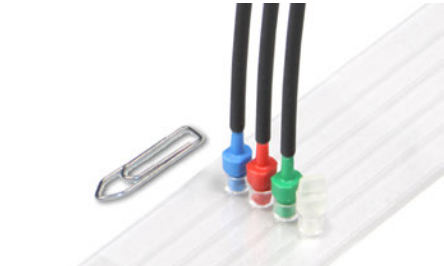
Fig. 346: PreSens SensorPlugs mounted on adjacent microfluidic channels
