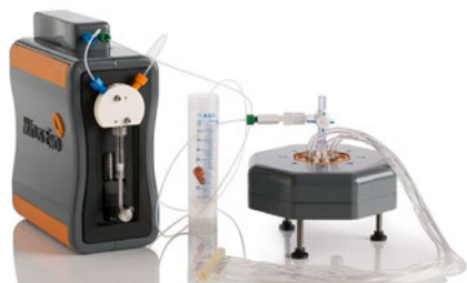
Fig. 759: Mirus Evo nanopump with MultiFlow8: controlled by PC software, VenaFlux assay (included)
