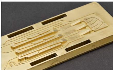
Fig. 898: Mold insert realized using ultraprecision mechanical machining
