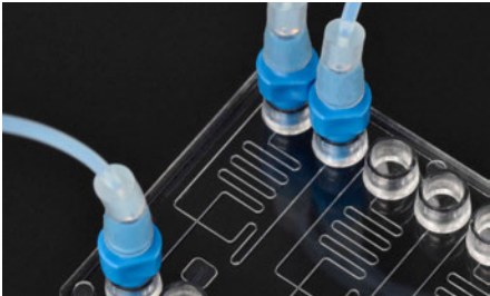
Fig. 265: Droplet generator Fluidic 440 – droplet size variation - interfaced with Mini Luer to fluid connectors and tubing
