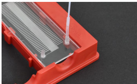
Fig. 690: PTFE tubing interconnected via silicone sleeve to the olive interface of a microfluidic device
