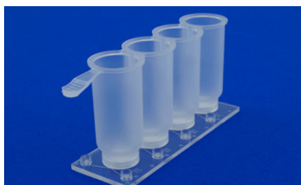
Fig. 1012: Transwell membrane chip Fluidic 219 with tank Fluidic 234 as fluid reservoir, TAB project number 2013 FE 9021
