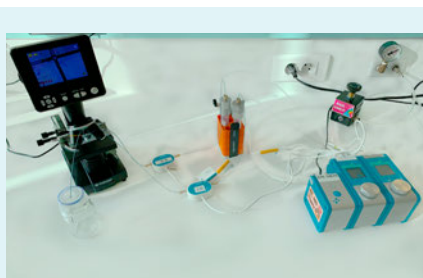
Droplet generation setup with droplet generator chip - on microscope - and Fluigent pressure-pump set-up
