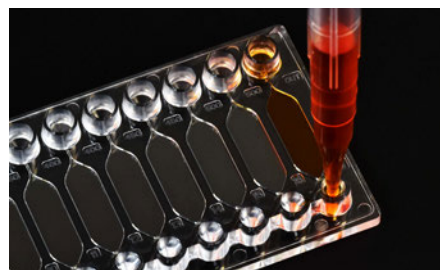
Fig. 95: Filling of the chip Fluidic 1495 using a conventional pipette
