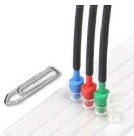
Fig. 519: Four PreSens' SensorPlugs on adjacent microfluidic channels
