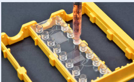
Fig. 855: Microfluidic chip with Luer interfaces filled with a standard syringe
