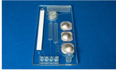
Fig. 983: Microfluidic chip with lateral flow strip based detection and implemented blister for liquid storage
