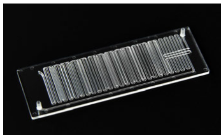
Fig. 722: 40 cycle continuous-flow PCR chip Fluidic 243
