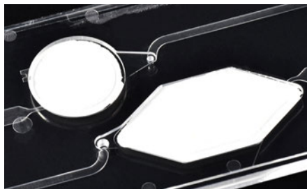
Fig. 313: Detail of the membrane chip Fluidic 783 with two separate plasma generation units - one round and one rhombic
