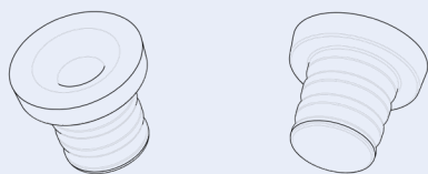
Fig. 605: Schematic drawing male Luer plunger with ripped surface Fluidic 1539
