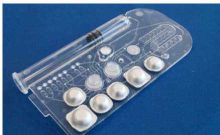
Fig. 1004: Integrated microfluidic chip for the detection of viral pathogens in the food supply chain, FP7 project EDEN, No. 313077
