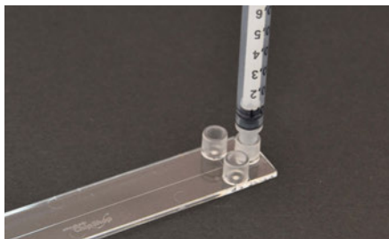
Fig. 67: Cross-shaped channel chip with female Luer interface and a syringe as male counterpart
