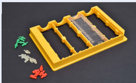
Fig. 874: Droplet generator Fluidic 285 placed in handling frame
