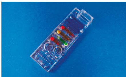
Fig. 964: Hybrid chip for immunoassays with electrochemical detection, realized within the EU-FP6 project "SmartHEALTH", No. 016817
