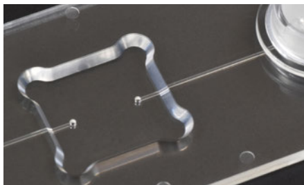
Fig. 492: Detail of the sensor integration area on Fluidic 673 without sensor
