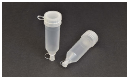
Fig. 677: Sampling vessel a total volume of 6.5 ml
