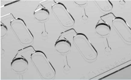
Fig. 375: Detail of the suspension cell chip Fluidic 1471 with inlet (through hole), circular cell cultivation chamber and downstream waste reservoir (oval chamber)
