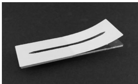
Fig. 464: Straight channel chip 268 with double-sided adhesive tape
