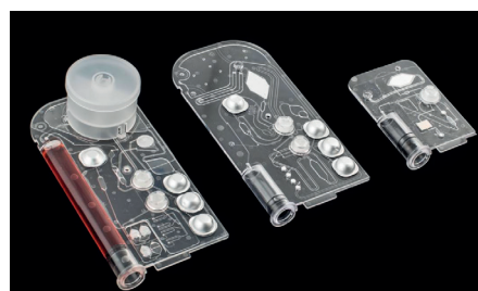
Sophisticated lab-on-a-chip devices with integrated membranes.
