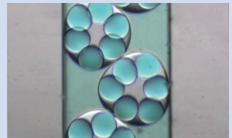
W/O/W (water in oil in water) droplets made possible through emulsifiers, i.e. surfactant in the oil phase
