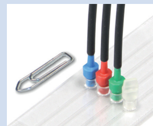
Four PreSens SensorPlugs mounted on adjacent microfluidic channels
