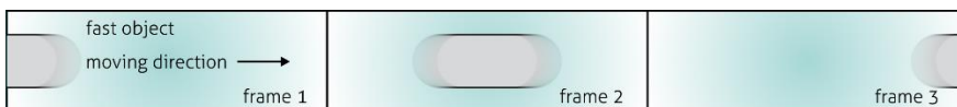
Figure 1: Standard video microscopy. Low frame rates don't allow high resolution motion tracking. Very strong motion blurring makes it impossible to determine particle shapes.
