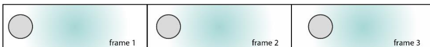
Figure 3: DeCellerator. High resolution in time and optimal imaging without motion blurring through synchronized pulsed illumination.
