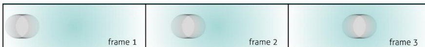
Figure 2: Fast video microscopy with standard illumination. Finer resolution in time, but motion blurring affects/hinders image analysis. Shorter exposure times can reduce motion blurring in exchange for worse signal to noise ratio.
