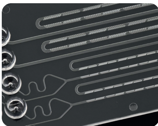
Fig.5: Channel structures of the chip
