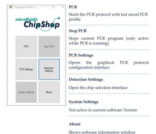
**Attention!** Clicking on the "Stop PCR" button will immediately interrupt the PCR protocol; the last set temperature will be maintained!
