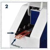
**2** Open the chip holder by pulling the chip locking lever out to the left. Insert the chip by sliding it below the guide rails.
