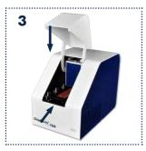
**3** Push the chip into the final position and close the chip locking lever by pushing it in. Close the lid.
