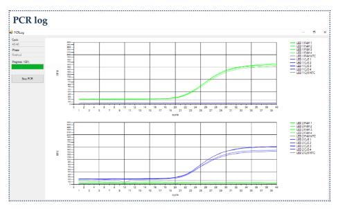
Two charts show the results of the fluorescence signals during the PCR. One chart displays the result for detection channel 1 (Fluo 1) the other chart displays the results for detection channel 2 (Fluo 2); all selected chambers of one detection channel are displayed in the same chart.
