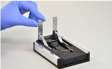
Fig. 463: Layout LOC HP/CCI 1 – Handling frame for chips in the format of a microscope slide
