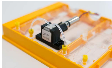
Fig. 691: CPP1 pump mounted on a handling frame via a holder (black) and connected to chips in slide format
