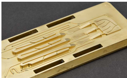
Fig. 788: Mold insert realized using ultraprecision mechanical machining
