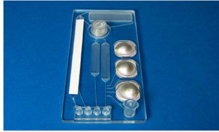
Fig. 854: Microfluidic chip with lateral flow strip based detection and implemented blister for liquid storage
