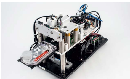
Fig. 891: Stratos breadboard unit – operating molecular, immunological and clinical chemistry assays
