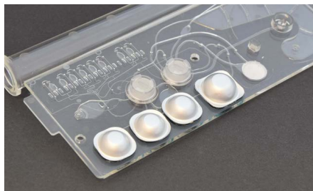
Fig. 528: Blister pouches of different volumes integrated in a complex microfluidic chip
