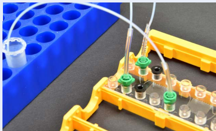
Fig. 753: Close unused fluid ports on chip with red Luer plugs
