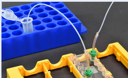
Fig. 752: Insertion of the Luer with tubings in fluid exit of the chip and connection of tube with sampling vessel
