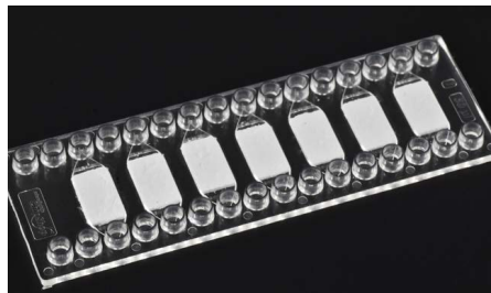
Fig. 890: Membrane for nucleic acid isolation within a chamber chip
