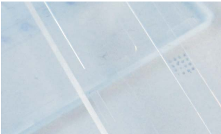
Fig. 142: Waste chamber chip – transparent with spotted probes
