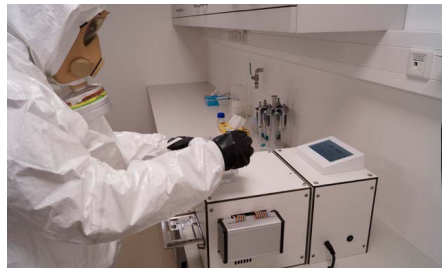
Fig. 874: Multisense Chip Analyzer: Demonstration of detection of airborne bacterial pathogens, FP7 project Multisense Chip, No. 261810
