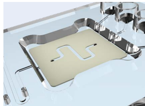
Fig. 403: Double-sided adhesive tape gasket – curved channel
