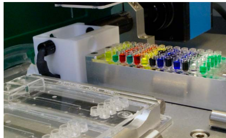
Fig. 204: 65-well chip used as source plate in spotter
