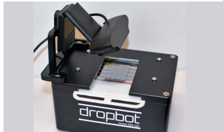
Fig. 632: DropBot instrument for manipulation and read-out
