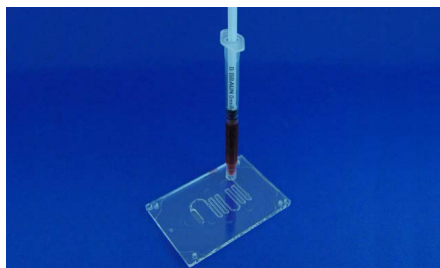
Fig. 851: Boyle-Marriott PCR chip for ultrafast PCR, design: IMM, realized within the FP 7 project "CD-Medics", No. 216031
