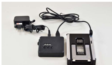
Fig. 627: Complete setup of the Lab-on-a-Chip Cell Culture Incubator – LOC CCI 1 with temperature control unit
