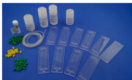
Fig. 708: ChipGenie® edition P starter kit 3 – DNA extraction from whole blood
