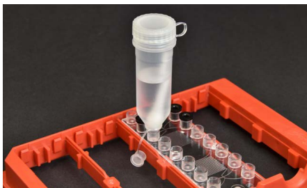
Fig. 572: Sampling vessel prefilled with buffer and inserted swab
