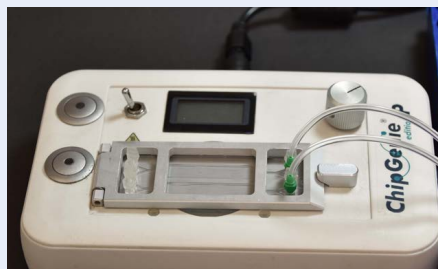
Fig 771: Chip inserted into ChipGenie® edition P instrument and installed connectors with silicone sleeve and PTFE tubing.
