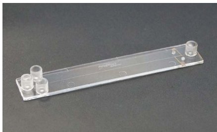
Fig. 67: Cross-shaped channel chip with electrodes for contactless conductivity detection
