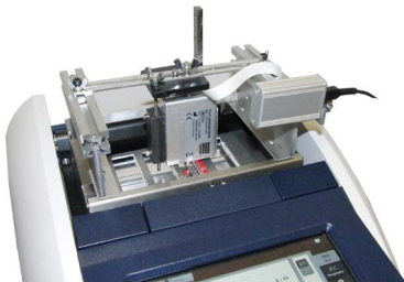
Fig. 722: Implementation of low-volume real-time PCR on chip – Chip on breadboard instrument
