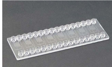
Fig. 241: Droplet generator – Similar chip layout for both Fluidic 440 and Fluidic 947
