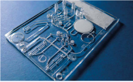
Fig. 837: Hybrid chip for immunoassays with plasma generation unit for electrochemical detection, realized within EU-FP6 project "SmartHEALTH", No. 016817
