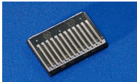
Fig. 860: Microfluidic chip realized for CARE-MAN - Health-CARE by biosensor Measurement and Networking, FP 6, NMP4-CT-2006-017333
