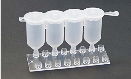
Fig. 556: Tank with cap for pneumatic actuation
