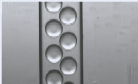
Fig. 769: Droplets generated on chip
