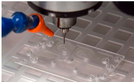
Fig. 784: Milling of various design features using a standardized interface platform
