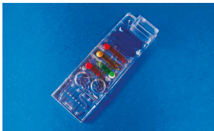
Fig. 835: Hybrid chip for immunoassays with electrochemical detection, realized within the EU-FP6 project "SmartHEALTH", No. 016817
