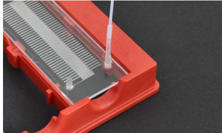
Fig. 580: PTFE tubing interconnected via silicone sleeve to the olive interface of a microfluidic device
