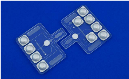
Fig. 879: Immunoassay-Chip, BMBF-Project HandyLoC, FKZ 13N13714
