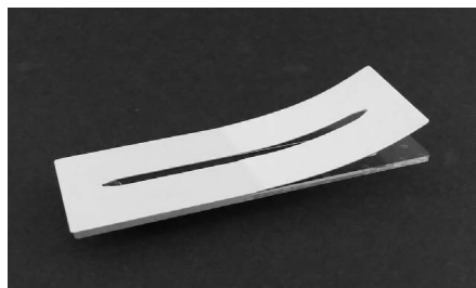
Fig. 392: Straight channel chip 268 with double-sided adhesive tape
