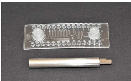
Fig. 376: Turning valve test chip with manual turning valve actuator
