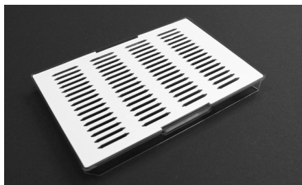
Fig. 387: Titer-plate sized microfluidic device for customization
