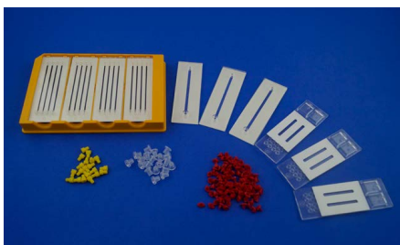
Fig. 715: DNA hybridization / microarray starter kit - spotting by customer
