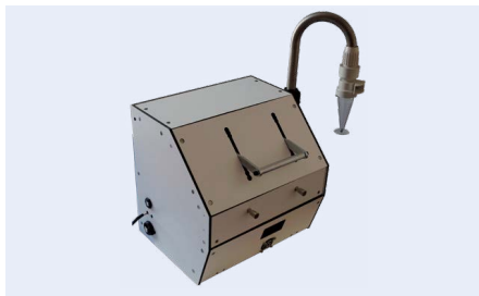
Fig. 863: Breadboard system: Electrochemical immunoassay system for air sample analysis, FP7 project Multisense Chip, No. 261810
