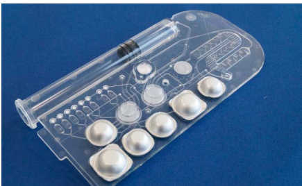
Fig. 875: Integrated microfluidic chip for the detection of viral pathogens in the food supply chain, FP7 project EDEN, No. 313077
