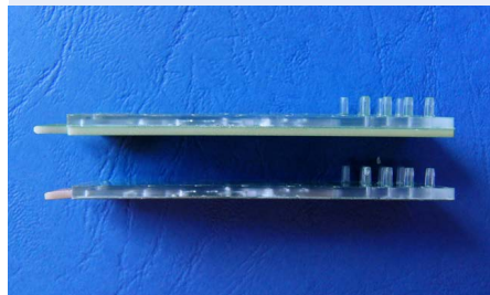
Fig. 844: Microfluidic chip coupled to conventional (top) and flex (bottom) PCBs, realized within the BMBF-project "SafeIS", FKZ 0315574C
