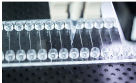
Fig. 635: instrumentTWO-300P spotting in microfluidic devices DNA-Array embedded in a microfluidic channel
