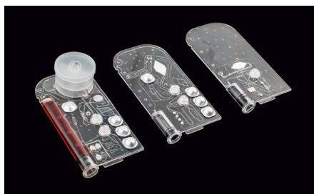
Fig. 893: Cartridges for the detection of tuberculosis, early HIV infection, and liver function (from left to right)
