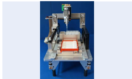
Fig. 858: Merger of standard liquid handling and lab-on-a-chip technology – LOC pipettor & xy-stage for optical read out, TAB project No. 2011 FE 9023
