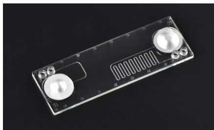
Fig. 378: Blister test chip Fluidic 289 with attached blister pouches
