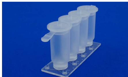
Fig. 884: Transwell membrane chip Fluidic 219 with tank Fluidic 235 as fluid reservoir, TAB project number 2013 FE 9021
