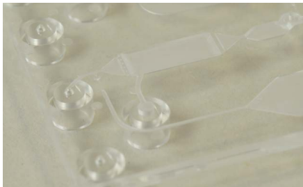
Fig. 785: Details of channels and chambers produced by milling a thermoplastic polymer platform
