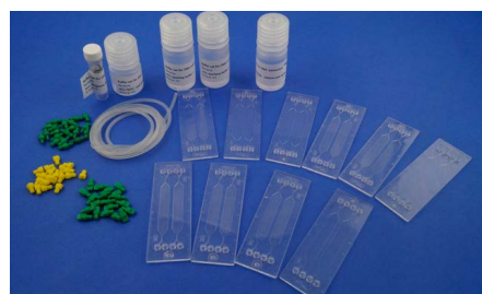
Fig. 709: ChipGenie® edition P starter kit 5 – DNA extraction from bacterial suspension
