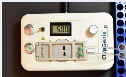
Fig. 773: ChipGenie® edition P instrument with washing buffer inside the rhombic chamber.
