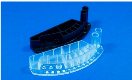
Fig. 859: Chip cuvette for frit-based immunoassays, realized within the BMBF project IFSA, FKZ 16SV5417
