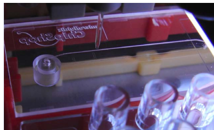
Fig. 637: instrument TWO-300P spotting in microfluidic devices DNA-Array embedded in a microfluidic channel
