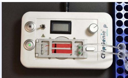
Fig 772: ChipGenie® edition P instrument with a blood sample inside the rhombic chamber. The magnetic beads, migrating through the chambers, are visible as black bars.
