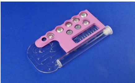
Fig. 881: Real-time PCR chip for B-agent detection, Horizon 2020 project, No. 700264
