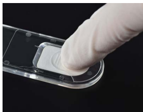
Fig. 901: Sample uptake via active finger pump
