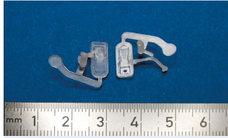
Fig. 838: Two component microinjection molding – Device for agglutination based assays, realized within the BMBF project FASAMOS, FKZ 02PC2001
