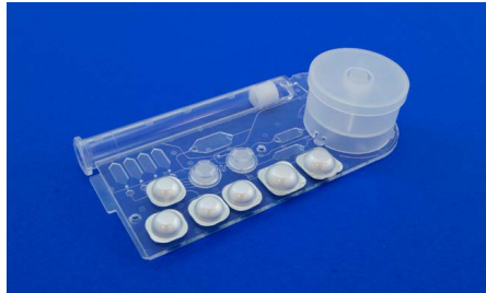
Fig. 880: Immunoassay-Chip for mycotoxine analysis, BMBF-Project Kombispec, FKZ 13N13757
