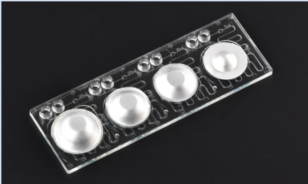
Blister test chip Fluidic 1021 with blister pouches of various volumes. Each blister is associated to an appropriate metering system
