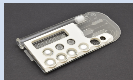
A sophisticated lab-on-a-chip device with mounted blister, which are protected by a cover from unintentional actuation
