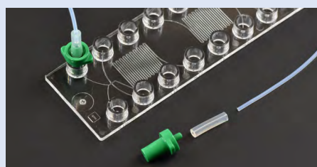
Assembly of a Luer fluid connector, silicone sleeve and PTFE tubing in Luer port on a disassembled connector setup
