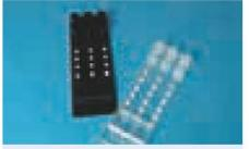
Fig. 240: IFSA 1 Immunoassay Chip – Equipped for three different samples with two measurement frits, one positive and one negative control frit
