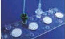
Fig. 292: Male Luer fluid connector with olive interface mounted on chip
