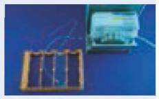
Fig. 487 Chip with olives connected via tubes to a peristaltic pump
