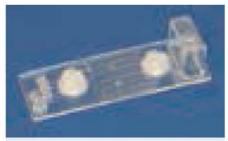
Fig. 233: Assay chip 2 – Fluidic 292 with embedded DNA array
