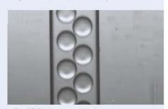
Fig. 497: Droplets generated on chip
