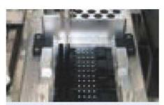
Fig. 389: Chips in microtiter sized handling frame placed in ChipGenie® edition I instrument
