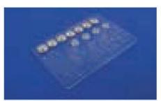
Fig. 586: Integrated microfluidic chip with complete sample preparation for miRNA analysis, BMBF project MRA, FKZ 0316078A
