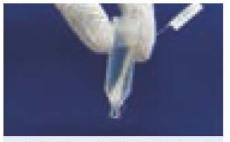
Fig. 329: Sampling vessel prefilled with buffer and inserted
