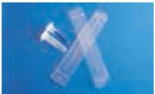
Fig. 66: Cross-shaped channel chips with through holes and electrodes
