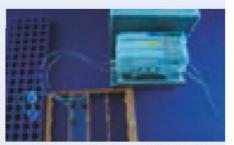
Fig. 481: Connection of the chip via the PTFE tube with the pump
