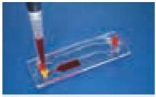
Fig. 276: Example of a Mini Luer to pipette adapter in use with a Rhombic Chamber chip
