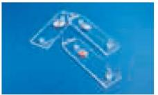
Fig. 301: Blister pouches integrated in a microfluidic chip
