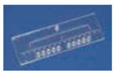
Fig. 580: One sample – 10 reactions: 0.5  $\mu$ l volume PCR chip, FP 7 project Multisense Chip, No. 261810
