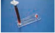
Fig. 278: Example of a Mini Luer to Luer adaptor in use with a Rhombic Chamber chip
