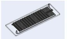
Fig. 367: Schematic drawing of 40 cycle continuous-flow PCR chip 243
