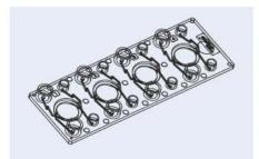
Fig. 168: Schematic drawing of cross-flow membrane chip Fluidic 398
