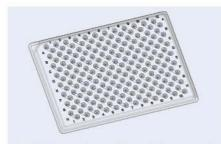
Fig. 33: Schematic drawing of the microfluidic microtiter plate top view – Fluidic  $600-150~\mu m$  channel depth
