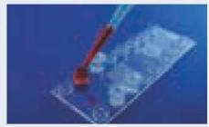
Fig. 473: Microfluidic chip with Luer interfaces filled with a pipette and interfaces used as rese voir
