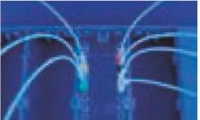
Fig. 128: Droplet generator chip Fluidic 285 in evaluation set-up
