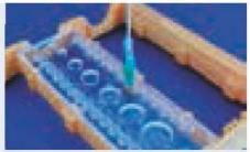
Fig. 467: Insertion of the Mini Luer with tubings in fluid entrance of the chip
