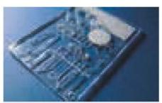
Fig. 556: Hybrid chip for immunoassays with plasma generation unit for electrochemical detection, realized within EU-FP6 project "SmartHEALTH", No. 016817
