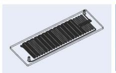
Fig. 150: Schematic drawing of 40 cycle continuous-flow PCR chip Fluidic 243
