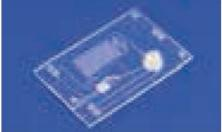
Fig. 589: Cartridge for CTC isolation and lysis. Realized within the EU-FP7 project "CanDo", project number: 610472
