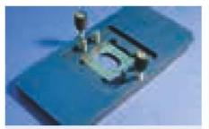
Fig. 258: MicCell support for 22x22 Channel Plates, to be placed in an inverted microscope via an adapter plate (not shown)
