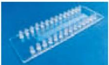
Fig. 364: 36-cycle continuous-flow PCR chip
