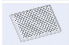
Fig. 35: Schematic drawing of the microfluidic microtiter plate top view – Fluidic 627 – 600  $\mu m$  channel depth
