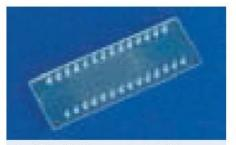
Fig. 147: Field flow fractionation chip Fluidic 159
