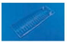
Fig. 362:15-cycle continuous-flow PCR-chip
