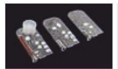
Fig. 600: Cartridges for the detection of tuberculosis, early HIV infection, and liver function (from left to right)
