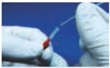
Fig. 335: PTFE tube connected via silicone sleeves to Mini Luer fluid connector
