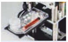
Fig. 599: microfluidic ChipShop's tuberculosis cartridge placed in the chip loader
