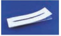
Fig. 446: Straight channel chip 268 with double-sided adhesive tape
