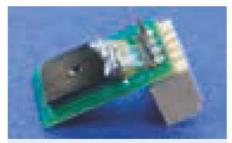
Fig. 398: PV6 hydrogel-containing silicon chip on a printed circuit board (top view)
