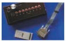
Fig. 385: Dielectrophoresis system DEP consisting of high frequency signal generator DEP1, microfluidic chip DFC1 and connecting cable
