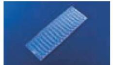
Fig. 461: Microfluidic platform with through holes as fluidic interface
