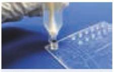
Fig. 328: Sampling vessel with septum on piercing interface
