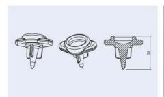
Fig. 273: Mini Luer plug – low volume displacement plug
