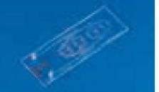
Fig. 555: Cell culture chips with integrated thin film electrodes, realized within the BMBF-Project "HepaChip", FKZ 01GG0728
