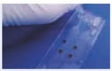
Fig. 498: Chip for  $120 \, \mu l$  sample volume with ready-made beads
