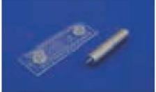
Fig. 218: Turning valve test chip with manual turning valve actuator
