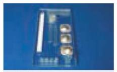
Fig. 320: DNA analysis chip with blister and integrated lateral flow strip
