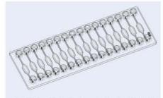
Fig. 91: Schematic drawing of reaction chamber chip Fluidic 585 – chamber volume 10  $\mu$ l
