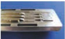
Fig. 514: Mold insert realised using ultraprecision mechanical machining
