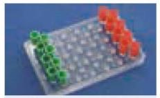
Fig. 596: Organ-on-chip device operated with hydrostatic fluid management, BMBF project HepoChip, FKZ 031A121D
