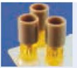
Fig. 295: Cross-shaped channel chip with three bonded port connectors and three chip reservoirs
