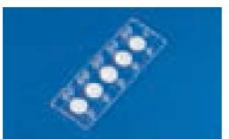
Fig. 552: Hybrid chip consisting of polymer and filters for plasma generation
