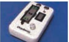
Fig. 378: ChipGenie® edition P instrument with bead-filled sample-prep chip
