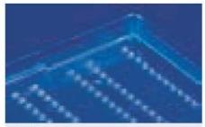
Fig. 31: Microfluidic titer plate
