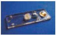
Fig. 575: Particle counting chip with integrated turning valve and staining solution, TAB project No. 2009 FE 0134
