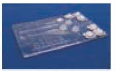
Fig. 592: Integrated microfluidic chip for the detection of bacterial pathogens, FP7 project Multisense Chip, No. 261810
