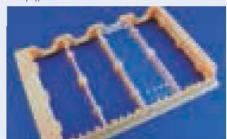
Fig. 484: Microfluidic chip with olive interfaces inserted in a microfluidic chip handling frame
