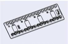
Fig. 57: Schematic drawing rhombic chamber chip
