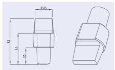
Fig. 103: Schematic drawing of a Mini Luer plug
