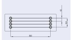
Fig. 13: Schematic drawing of the four-channel Mini Luer chip family
