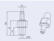
Fig. 99: Schematic drawing of a Mini Luer connector
