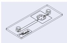
Fig. 23: Schematic drawing of a straight channel chip with additional large chamber
