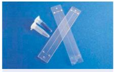
Fig. 40: Cross-shaped channel chips with through holes and electrodes
