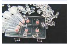
Fig. 192: PCR chip with integrated freez-dried master mix
