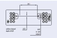
Fig. 61: Detail of droplet generator 0162
