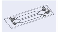
Fig. 47: Schematic drawing of the rhombic chamber chip
