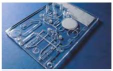
Fig. 198: Hybrid chip for immunoassays with plasma generation unit for electrochemical detection, realized within EU-FP6 project "SmartHEALTH", No. 016817
