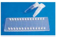
Fig. 167: Example of microscopy slide olive platform with 28 olive fittings
