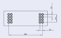
Fig. 174: Microscopy slide Mini Luer platform – version with 16 fluidic interfaces on the short edges
