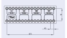
Fig. 44: Detail of H-shaped channel chip
