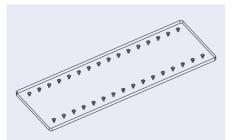
Fig. 162: Microscopy slide through-hole platform – version with 32 fluidic interfaces
