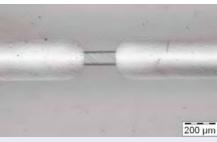
Fig. 143: Microscopy image of electrodes over microchannel
