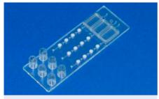
Fig. 202: Microfluidic chip for immunoassay applications with reagent reservoirs and antibody-coated frits for three assays, realized within the BMBF project IFSA, FKZ 16SV5417
