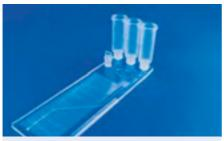
Fig. 109: Tanks mounted on a microfluidic chip
