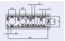
Fig. 60: Rhombic chamber chip – chamber volumes: 60  $\mu l,$  40  $\mu l,$  2 x 20  $\mu l,$  2 x 10  $\mu l$
