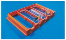
Fig. 46: Rhombic chamber chip in handling frame connected to PCR chip
