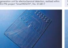
Fig. 200: Sample-in-result-out DNA-analysis chip, realized within the BMBF project ChipFlussPCR, FKZ 13N9556
