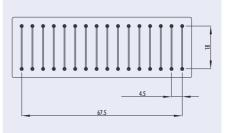
Fig. 7: Schematic drawing of the 16-channel through-hole chip family
