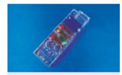
Fig. 196: Hybrid chip for immunoassays with electrochemical detection, realized within the EU-FP6 project "SmartHEALTH", No. 016817
