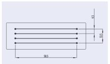
Fig. 6: Details of the four-channel through-hole chip family
