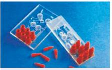
Fig. 108: Prototyped analytical platforms with Upchurch Nanoports
