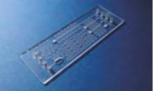
Fig. 201: Microfluidic chip for a complete SELEX-cycle, realized within the ETB project Artamis, FKZ 03139428
