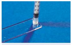
Fig. 32: Cross-shaped channel chip with female Luer interface and a syringe as male counterpart
