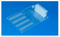
Fig. 203: Sample-in-result-out DNA-analysis chip with hybridisation zone for optoelectronic read-out, realized within the project PatholD Chip, A-102-RT-GC
