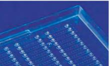
Fig. 22: Microfluidic titer plate with spotted probes
