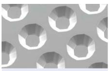
Fig. 72: Nanotiter plate – well detail
