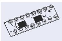
Fig. 81: Schematic drawing of diffusion mixer
