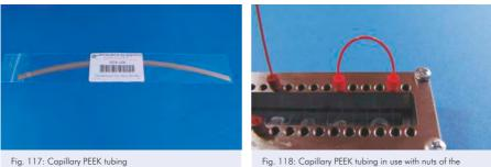
Fig. 118: Capillary PEEK tubing in use with nuts of the Upchurch Nanoport set in combination with a chip adapter frame
