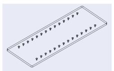
Fig. 161: Microscopy slide through-hole platform – version with 28 fluidic interfaces
