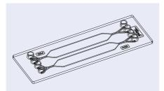
Fig. 146: Schematic drawing of the rhombic chamber chip
