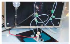
Fig. 154: MicCell FP-1-1-standard Fluid Processor. Foreground: MicCell with hydrogel valve in its blue support and black adapter plate
