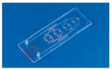
Fig. 197: Cell culture chips with integrated thin film electrodes, realized within the BMBF-Project "HepaChip", FKZ 01GG0728
