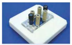
Fig. 96: Casting Station 22 mm x 22 mm. Top: assembled, including channel spacers (brown)
