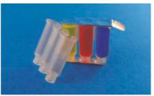
Fig. 112: Filled tanks sealed with alumina foil
