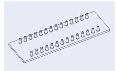
Fig. 165: Microscopy slide olive platform – version with 28 fluidic interfaces
