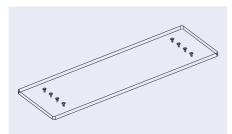
Fig. 160: Microscopy slide through-hole platform  $-\,version$  with eight fluidic interfaces
