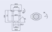
Fig. 105: Schematic drawing of the Luer Lok compatible adapter
