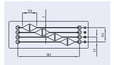
Fig. 85: Schematic drawing of weir chip
