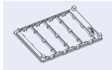
Fig. 123: Schematic drawing of handling frame with flat skirt
