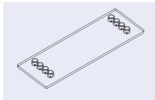
Fig. 172: Microscopy slide Mini Luer platform – version with eight fluidic interfaces
