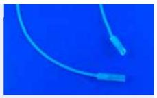
Fig. 450: Short pieces of silicone tubes connected with PTFE tube
