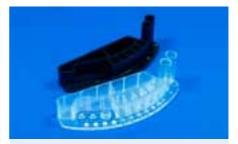
Fig. 545: Chip cuvette for frit-based immunoassays, realized within the BMBF project IFSA, FKZ 16SV5417
