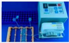
Fig. 436: Connection of pump via a PTFE tube with a liquid reservoir
