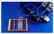
Fig. 458: Side ports for oil phase of the droplet generator chip connected to the pump
