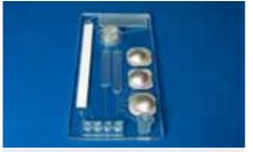
Fig. 284: DNA analysis chip with blister and integrated lateral flow strip
