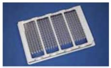
Fig. 306: Handling frame for microscopy slide format chips to fit 384 well positions of a microtiterplate – fitting with 384 well plate readers
