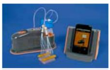
Fig. 366: Kima pump, controlled by iPod Touch
