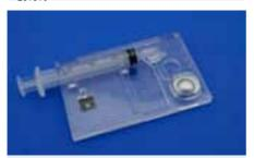
Fig. 554 Selective cell counting chip for hematology, BMBF project MrCyte, FKZ 13N12018
