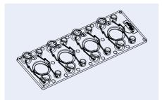
Fig. 154: Schematic drawing of cross-flow membrane chip 398
