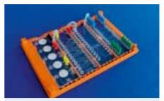
Fig. 305: Handling frame with flat skirt with different chip types connected with each other
