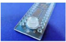
Fig. 531: Fluidic chip with rotary valve
