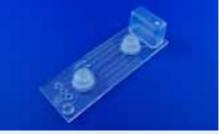
Fig. 537: Enyzme-assay development chip, realized within the FP 7 project Multisense Chip, No. 261810
