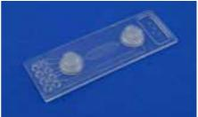
Fig. 202: Assay chip 3 – Fluidic 490 with central reaction chamber and integrated turning valve for fluid actuation
