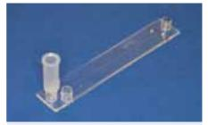
Fig. 277: 500  $\mu$ l single tank mounted on Luer interface
