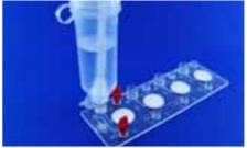
Fig. 289: Sampling vessel prefilled with buffer and inserted
