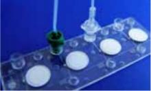
Fig. 260: Male Luer fluid connector with olive interface mounted on chip
