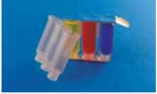
Fig. 271: Filled tanks sealed with alumina foil
