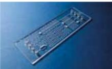
Fig. 525: Microfluidic chip for a complete SELEX-cycle, realized within the ETB project Artamis, FKZ 03139428
