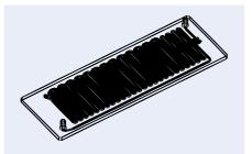
Fig. 136: Schematic drawing of 40 cycle continuous-flow PCR chip Fluidic 243
