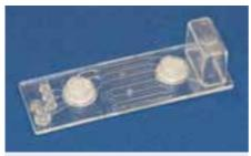
Fig. 199: Assay chip 2 – Fluidic 292 with embedded DNA array
