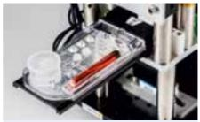
Fig. 557: microfluidic ChipShop's tuberculosis cartridge placed in the chip loader
