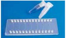
Fig. 490: Example of microscopy slide olive platform with 28 olive fittings
