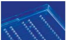
Fig. 26: Microfluidic titer plate with spotted probes
