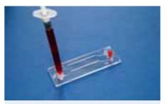
Fig. 246: Example of a Mini Luer to Luer adaptor in use with a Rhombic Chamber chip
