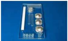
Fig. 539: Microfluidic chip with lateral flow strip based detection and implemented blister for liquid storage
