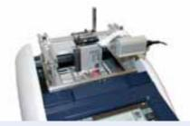
Fig. 414: Implementation of low-volume real-time PCR on chip – Chip on breadboard instrument
