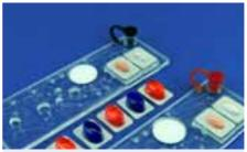
Fig. 533: Immunoassay chip with plasma generation unit and blister pouches  $\,$
