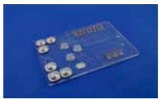
Fig. 552: Integrated microfluidic chip for the detection of bacterial pathogen on molecular and immunological level with integrated electrodes, FP7 project Multisense Chip, No. 261810
