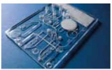
Fig. 522: Hybrid chip for immunoassays with plasma generation unit for electrochemical detection, realized within EU-FP6 project "SmartHEALTH", No. 016817
