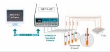
Fig. 373: Schematic set-up of Fluigent's MFCS™-EZ pressure-based flow controller with fluid reservoir and connection to the microfluidic device
