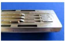
Fig. 479: Mold insert realised using ultraprecision mechanical machining
