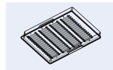
Fig. 23: Schematic drawing of the microfluidic titer plate
