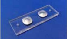
Fig. 285: Blister test chip with aluminum foil pouches
