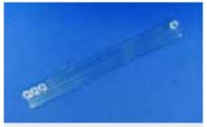
Fig. 50: Cross-shaped channel chip with Luer interfaces
