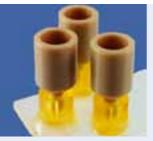
Fig. 263: Cross-shaped channel chip with three bonded port connectors and three chip reservoirs
