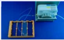
Fig. 452 Chip with olives connected via tubes to a peristaltic
