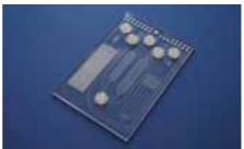
Fig. 547: Integrated microfluidic chip for continuous-flow PCR and parallel immunoassay, FP7 project Multisense Chip, No. 261810
