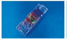
Fig. 520: Hybrid chip for immunoassays with electrochemical detection, realized within the EU-FP6 project "SmartHEALTH", No. 016817
