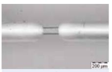
Fig. 338: Microscopy image of electrodes over microchannel
