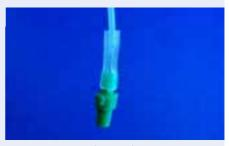
Fig. 431: Connection of Mini Luer fluid connector with mounted silicone sleeve with a PTFE tube
