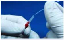
Fig. 299: PTFE tube connected via silicone sleeves to Mini Luer fluid connector
