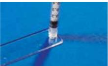
Fig. 44: Cross-shaped channel chip with female Luer interface and a syringe as male counterpart
