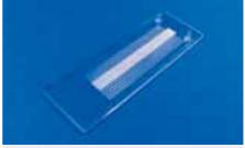
Fig. 330: 41-cycle continuous-flow PCR chip
