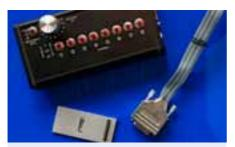
Fig. 349: Dielectrophoresis system DEP consisting of high frequency signal generator DEP1, microfluidic chip DFC1 and connecting cable
