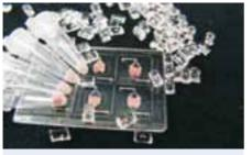
Fig. 516: PCR chip with integrated freez-dried master mix
