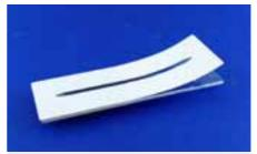
Fig. 411: Straight channel chip 0268 with double-sided adhesive tape
