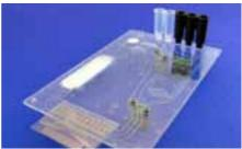
Fig. 535: Serology test chip for the detection of coeliac disease, realized within the FP 7 project "CD-Medics", No.216031
