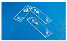
Fig. 269: Blister pouches integrated in a microfluidic chip
