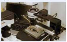
Fig 473: Lab-on-a-Chip Cell Culture Incubator – LOC CCI 1 during use on microscope stage
