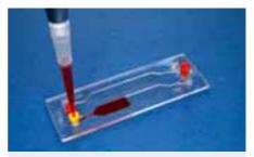
Fig. 244: Example of a Mini Luer to pipette adaptor in use with a Rhombic Chamber chip
