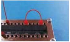
Fig. 297: Capillary PEEK tubing in use with nuts of the Upchurch Nanoport set in combination with a chip adapter frame
