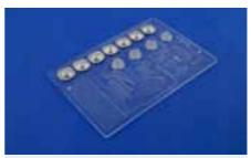
Fig. 553: Integrated microfluidic chip with complete sample preparation for miRNA analysis, BMBF project IMRA, FKZ 0316078A
