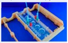
Fig. 434: Closed unused fluid ports on chip with red Mini Luer plugs
