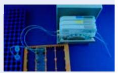
Fig. 446: Connection of the chip via the PTFE tube with the pump  $\,$
