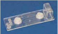
Fig. 198: Assay chip 2- Fluidic 292 with hybridization chamber and integrated turning valve for fluid actuation
