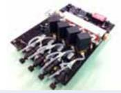
Fig. 372: OEM version of Fluigent's MFCS<sup>TM</sup>-EZ pressurebased flow controller for pre-industrial or industrial applications
