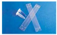
Fig. 60: Cross-shaped channel chips with through holes and electrodes
