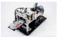
Fig. 556: Stratos breadboard unit – operating molecular, immunological and clinical chemistry assays
