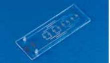
Fig. 521: Cell culture chips with integrated thin film electrodes, realized within the BMBF-Project "HepaChip", FKZ 01GG0728
