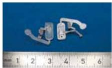
Fig. 523: Two component microinjection molding – Device for agglutionation based assays, realized within the BMBF project FASAMOS, FKZ 02PC2001
