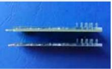
Fig. 529: Microfluidic chip coupled to conventional (top) and flex (bottom) PCBs, realized within the BMBF-project "SafelS", FKZ 0315574C
