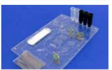
Fig. 534: HLA typing chip for the detection of coeliac disease, realized within the FP 7 project "CD-Medics", No. 216031
