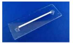
Fig. 22: One channel Luer chip with inserted lateral flow strip and spotted probes
