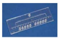
Fig. 546: One sample – 10 reactions: 0.5  $\mu$ l volume PCR chip, FP 7 project Multisense Chip, No. 261810
