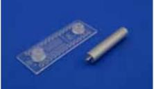
Fig. 190: Turning valve test chip with manual turning valve actuator
