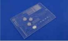
Fig. 551: Integrated microfluidic chip for the detection of bacterial pathogen on molecular and immunological level, FP7 project Multisense Chip, No. 261810
