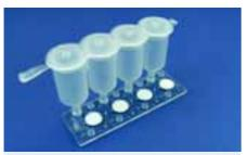
Fig. 530: Filtration chip with liquid reservoir
