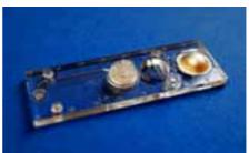
Fig. 541: Particle counting chip with integrated turning valve and staining solution, TAB project No. 2009 FE 0134
