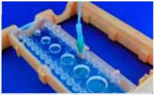
Fig. 432: Insertion of the Mini Luer with tubings in fluid entrance of the chip
