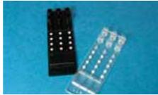
Fig. 208: IFSA 1 Immunoassay Chip – Equipped for three different samples with two measurement frits, one positive and one negative control frit
