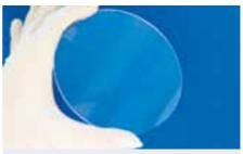
Fig. 316: 115 mm diameter wafer
