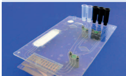
Fig. 403: Serology test chip for the detection of coeliac disease, realized within the FP 7 project "CD-Medics", No.216031
