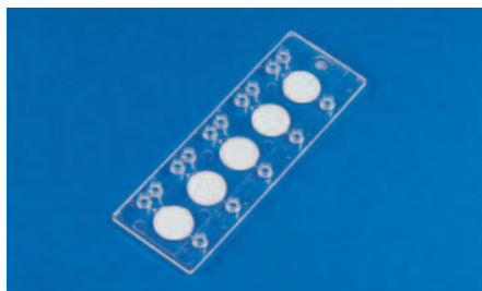
Fig. 386: Hybrid chip consisting of polymer and filters for plasma generation
