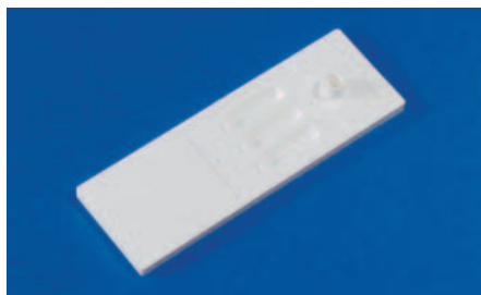
Fig. 382: Diagnostic platform with Luer connectors
