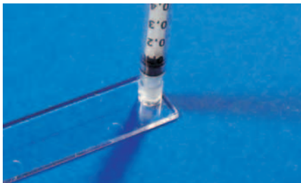
Fig. 40: Cross-shaped channel chip with female Luer interface and a syringe as male counterpart
