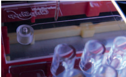
Fig. 286: DNA-array embedded in a microfluidic channel
