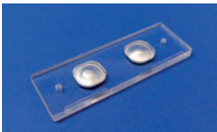
Fig. 202: Blister test chip with aluminum foil pouches
