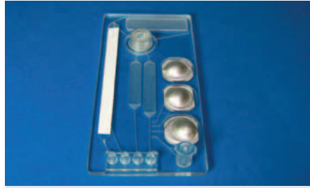
Fig. 407: Microfluidic chip with lateral flow strip based detection and implemented blister for liquid storage
