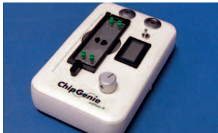
Fig. 249: ChipGenie® edition P instrument with bead-filled sample-prep chip
