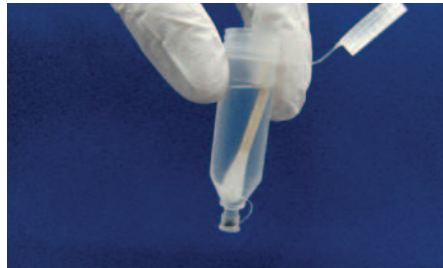
Fig. 210: Sampling vessel prefilled with buffer and inserted swab
