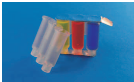
Fig. 190: Filled tanks sealed with alumina foil
