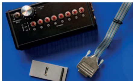
Fig. 256: Dielectrophoresis system DEP consisting of high frequency signal generator DEP1, microfluidic chip DFC1 and connecting cable
