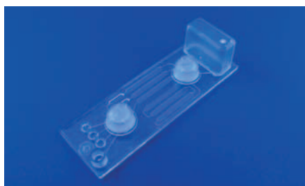
Fig. 405: Enzyme-assay development chip, realized within the FP 7 project Multisense Chip, No. 261810
