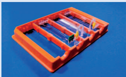
Fig. 324: Microfluidic chip with olive connected to different chip types
