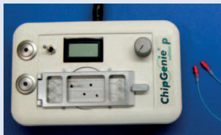
Fig 340: Chip inserted in ChipGenie® edition P
