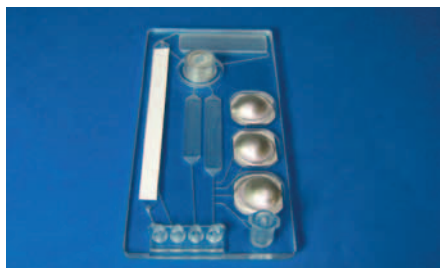
Fig. 201: DNA analysis chip with blister and integrated lateral flow strip
