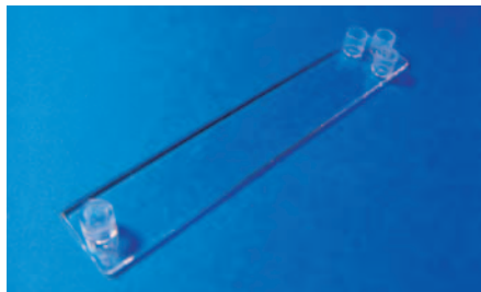
Fig. 39: Cross-shaped channel chip with Luer interfaces
