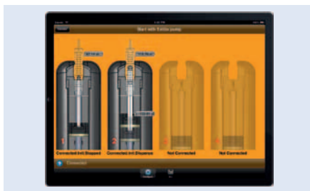
Fig. 269: iPad mini App for ExiGo pump showing sample volume to be dispensed from each pump
