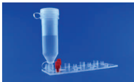
Fig. 205: Sampling vessel prefilled with liquid mounted on a chip
