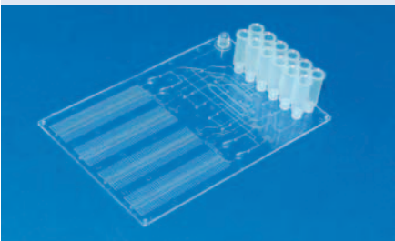
Fig. 396: Sample-in-result-out DNA-analysis chip with hybridisation zone for optoelectronic read-out, realized within the project PathoID Chip, A-102-RT-GC
