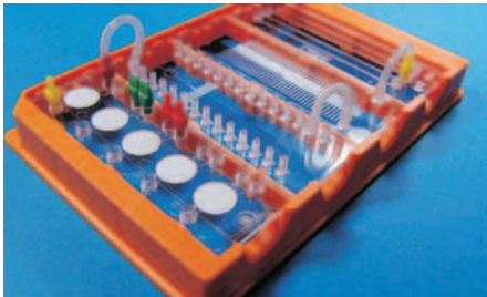
Fig. 220: Handling frame with different chip types connected with each other
