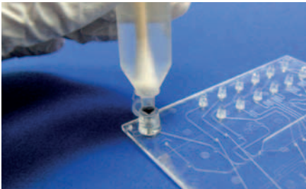
Fig. 209: Sampling vessel with septum on piercing interface on chip
