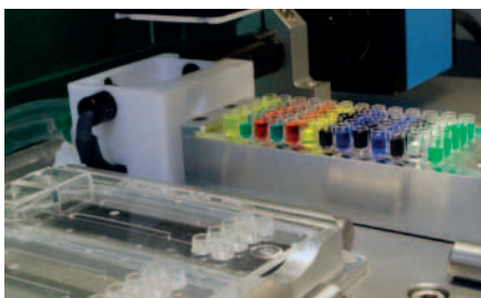
Fig. 105: 65-well chip used as source plate in spotter
