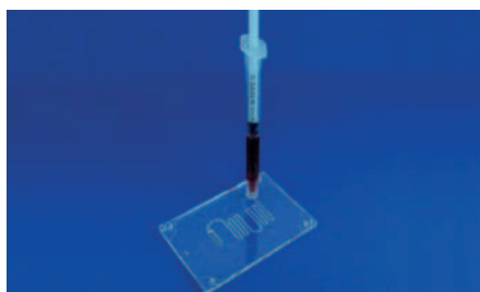
Fig. 404: Boyle-Mariotte PCR chip for ultrafast PCR, design: IMM, realized within the FP 7 project "CD-Medics", No. 216031
