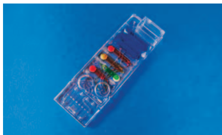
Fig. 388: Hybrid chip for immunoassays with electrochemical detection, realized within the EU-FP6 project "SmartHEALTH", No. 016817
