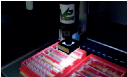
Fig. 285: Spotting in microfluidic devices – M2-Automation instrumentTWO in action
