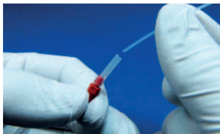
Fig. 216: PTFE tube connected via silicone sleeves to Mini Luer fluid connector
