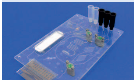
Fig. 402: HLA typing chip for the detection of coeliac disease, realized within the FP 7 project "CD-Medics", No. 216031
