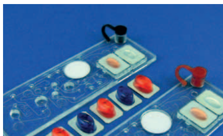
Fig. 401: Immunoassay chip with plasma generation unit and blister pouches
