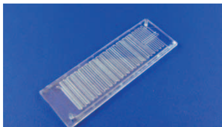
Fig. 97: 40 cycle continuous-flow PCR chip 0243
