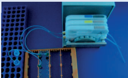
Fig. 322: Connection of the chip via the PTFE tube with the pump
