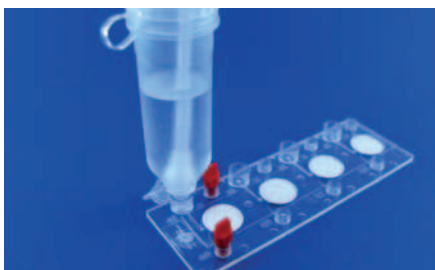
Fig. 206: Sampling vessel prefilled with buffer and inserted swab
