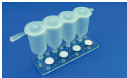
Fig. 398: Filtration chip with liquid reservoir
