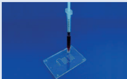
Fig. 313: Microfluidic chip with Luer interfaces filled with a standard syringe
