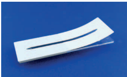
Fig. 292: Straight channel chip 0268 with double-sided adhesive tape
