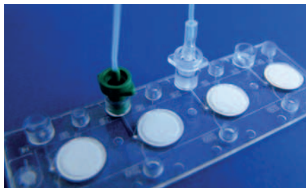
Fig. 179: Male Luer fluid connector with olive interface mounted on chip
