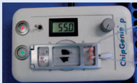
Fig. 342: Beads on chip during clean-up and elution
