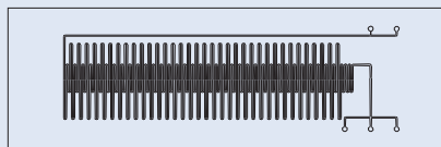
Fig. 236: Schematic drawing of 36-cycle continuous-flow PCR chip
