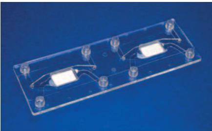
Fig. 410: Cell culture chip with integrated membrane, TAB project No. 2011 FE 9014
