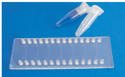
Fig. 359: Example of microscopy slide olive platform with 28 olive fittings
