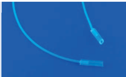
Fig. 326: Short pieces of silicone tubes connected with PTFE tube
