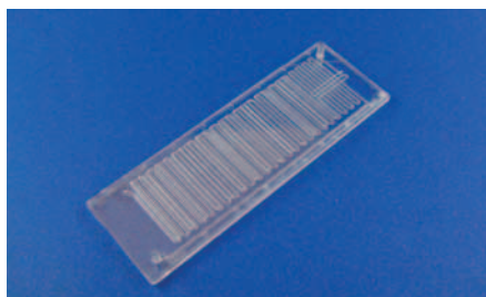
Fig. 241: 40 cycle continuous-flow PCR chip 0243
