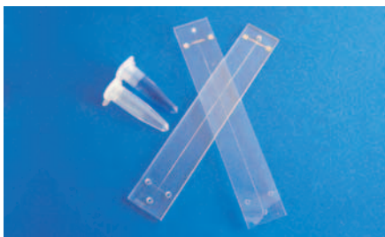
Fig. 56: Cross-shaped channel chips with through holes and electrodes
