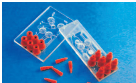
Fig. 181: Prototyped analytical platforms with Upchurch Nanoports
