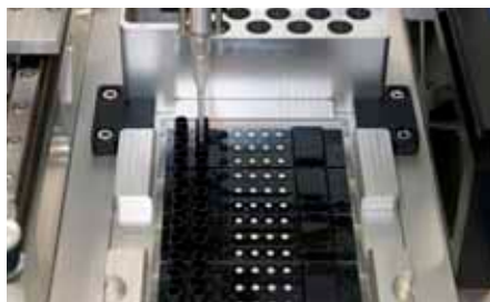
Fig. 299: Chips in microtiter sized handling frame placed in ChipGenie® edition I instrument
