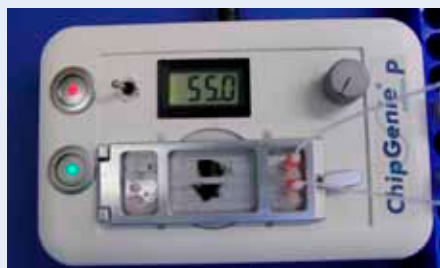
Fig. 398: Beads on chip during clean-up and elution
