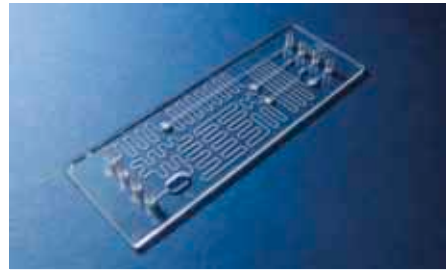
Fig. 455: Microfluidic chip for a complete SELEX-cycle, realized within the ETB project Artamis, FKZ 03139428
