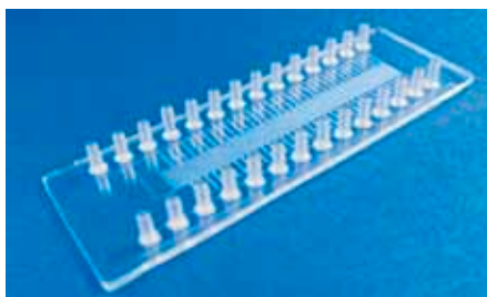
Fig. 274: 36-cycle continuous-flow PCR chip
