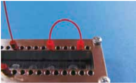
Fig. 245: Capillary PEEK tubing in use with nuts of the Upchurch Nanoport set in combination with a chip adapter frame
