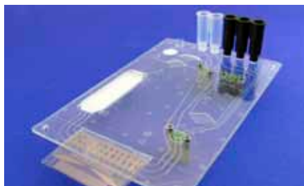
Fig. 465: Serology test chip for the detection of coeliac disease, realized within the FP 7 project "CD-Medics", No. 216031
