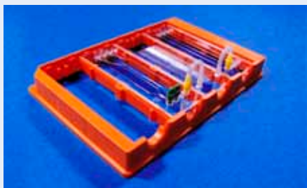
Fig. 380: Microfluidic chip with olive connected to different chip types
