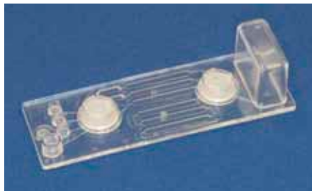
Fig. 153: Assay chip 2 with embedded DNA array
