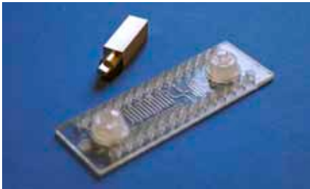
Fig. 148: Turning valve test chip with manual turning valve actuator
