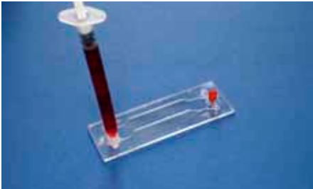
Fig. 194: Example of a Mini Luer to Luer adaptor in use with a Rhombic Chamber chip
