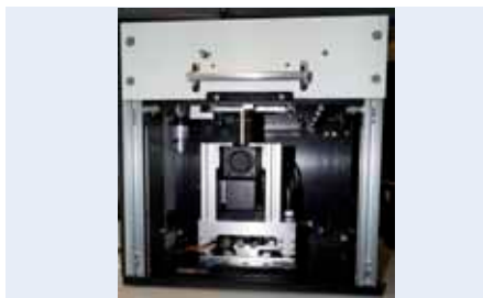
Fig. 479: Breadboard system: Lab-on-a-Chip instrument for optical read-out of immunoassays, TAB project LabChipLO
