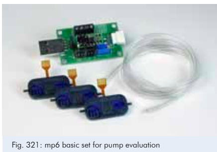
Fig. 321: mp6 basic set for pump evaluation
