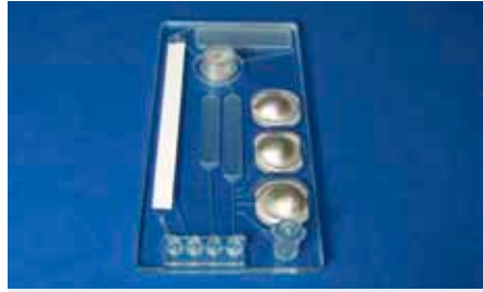
Fig. 469: Microfluidic chip with lateral flow strip based detection and implemented blister for liquid storage
