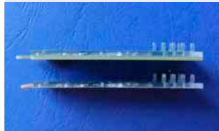
Fig. 459: Microfluidic chip coupled to conventional (top) and flex (bottom) PCBs, realized within the BMBF-project "SafeIS", FKZ 0315574C
