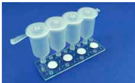
Fig. 460: Filtration chip with liquid reservoir
