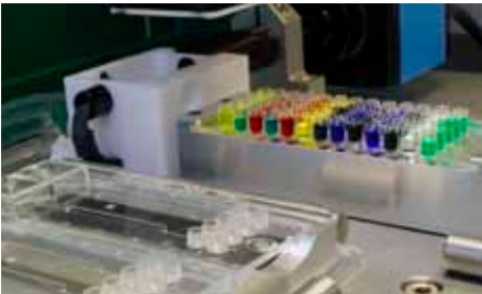
Fig. 109: 65-well chip used as source plate in spotter
