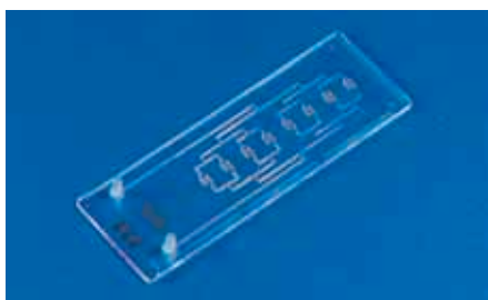
Fig. 451: Cell culture chips with integrated thin film electrodes, realized within the BMBF-Project "HepaChip", FKZ 01GG0728
