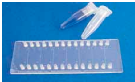
Fig. 421: Example of microscopy slide olive platform with 28 olive fittings
