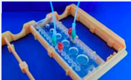
Fig. 366: Closed unused fluid ports on chip with red Mini Luer plugs
