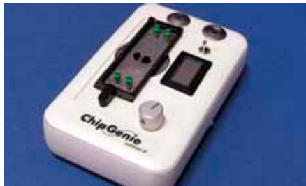
Fig. 288: ChipGenie® edition P instrument with bead-filled sample-prep chip
