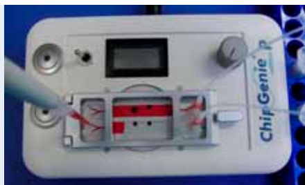
Fig 397: Chip and ChipGenie® edition P during sample loading
