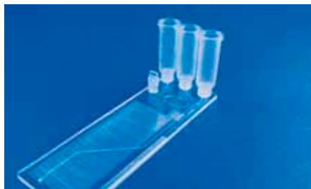
Fig. 216: Tanks mounted on a microfluidic chip
