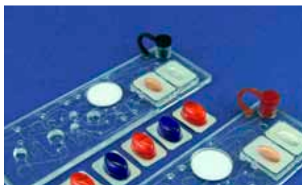
Fig. 463: Immunoassay chip with plasma generation unit and blister pouches
