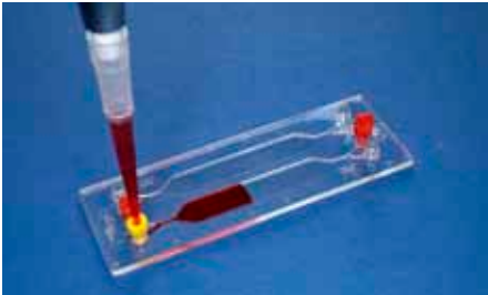
Fig. 192: Example of a Mini Luer to pipette adaptor in use with a Rhombic Chamber chip
