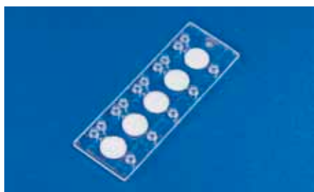
Fig. 448: Hybrid chip consisting of polymer and filters for plasma generation
