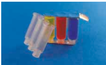
Fig. 219: Filled tanks sealed with alumina foil
