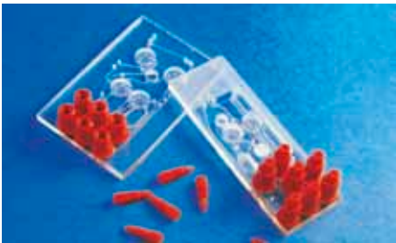
Fig. 210: Prototyped analytical platforms with Upchurch Nanoports
