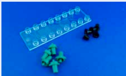
Fig. 371: Microfluidic chip with Luer interfaces with Luer fluid connectors and plugs
