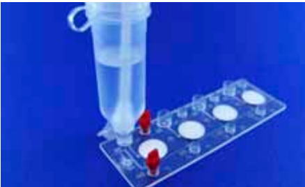
Fig. 237: Sampling vessel prefilled with buffer and inserted swab
