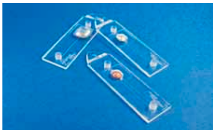
Fig. 217: Blister pouches integrated in a microfluidic chip
