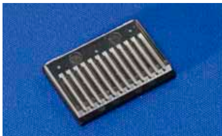
Fig. 480: Microfluidic chip realized for CARE-MAN - Health-CARE by biosensor Measurement and Networking, FP 6, NMP4-CT-2006-017333
