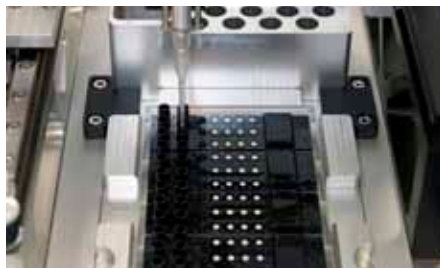
Fig. 164: IFSA 1 Immunoassay Chip in ChipGenie® edition I instrument
