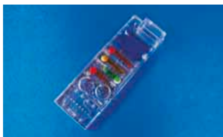
Fig. 450: Hybrid chip for immunoassays with electrochemical detection, realized within the EU-FP6 project "SmartHEALTH", No. 016817
