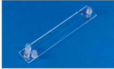
Fig. 58: Cross-shaped channel chip with electrodes for contactless conductivity detection
