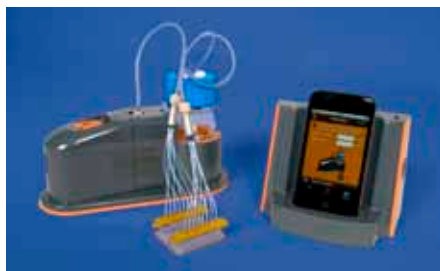
Fig. 311: Kima pump, controlled by iPod Touch
