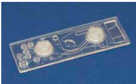
Fig. 150: Assay chip 1 with on-chip metering, mixing, reaction and detection chamber and two integrated turning valve
