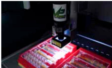
Fig. 336: Spotting in microfluidic devices – M2-Automation instrumentTWO in action
