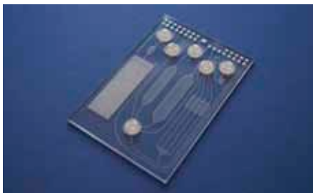
Fig. 477: Integrated microfluidic chip for continuous-flow PCR and parallel immunoassay, FP7 project Multisense Chip, No. 261810
