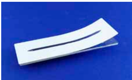
Fig. 343: Straight channel chip 0268 with double-sided adhesive tape
