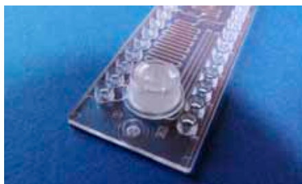
Fig. 242: Fluidic chip with embedded rotary valve
