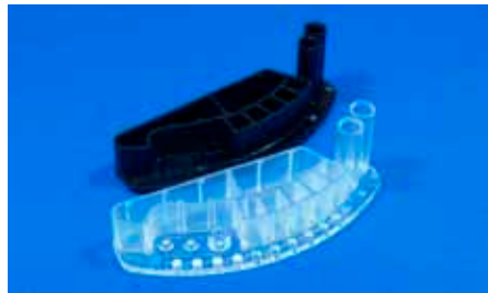
Fig. 475: Chip cuvette for frit-based immunoassays, realized within the BMBF project IFSA, FKZ 16SV5417
