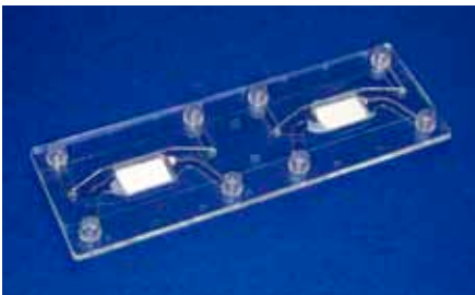
Fig. 472: Cell culture chip with integrated membrane, TAB project No. 2011 FE 9014
