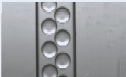
Fig. 394: Droplets generated on chip
