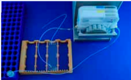
Fig. 385: Pump tube connected to reservoir vessel
