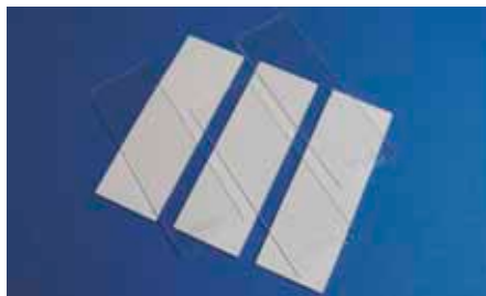
Fig. 266: Various polymeric substrates in the format of a microscopy slide
