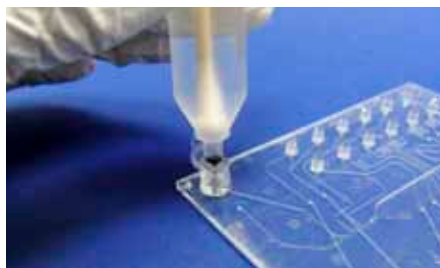
Fig. 240: Sampling vessel with septum on piercing interface on chip
