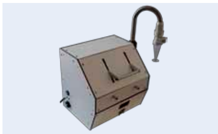
Fig. 478: Breadboard system: Electrochemical immunoassay system for air sample analysis, FP7 project Multisense Chip, No. 261810
