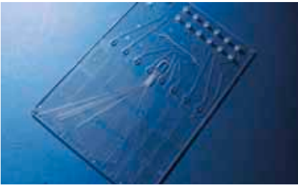
Fig. 454: Sample-in-result-out DNA-analysis chip, realized within the BMBF project ChipFlussPCR, FKZ 13N9556
