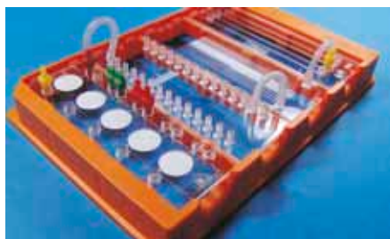
Fig. 251: Handling frame with different chip types connected with each other
