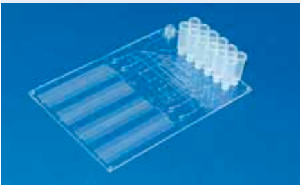
Fig. 458: Sample-in-result-out DNA-analysis chip with hybridisation zone for optoelectronic read-out, realized within the project PathoID Chip, A-102-RT-GC
