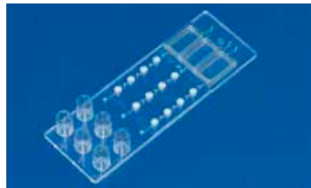
Fig. 457: Microfluidic chip for immunoassay applications with reagent reservoirs and antibody-coated frits for three assays, realized within the BMBF project IFSA, FKZ 16SV5417
