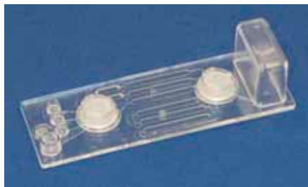
Fig. 152: Assay chip 2 with hybridization chamber and integrated turning valve for fluid actuation
