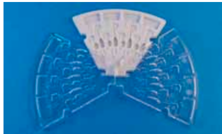
Fig. 443: Examples of pie slice plate chips. The chips were developed within the BMBF-Project "ZentriLab", FKZ 16SV2350.
