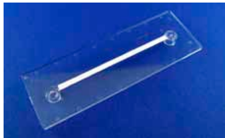
Fig. 22: One channel Luer chip with inserted lateral flow strip and spotted probes
