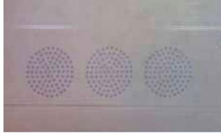
Fig. 34: Spotted probes (diameter 80 \mu\text{m} ) in straight channel chip 0272
