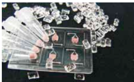
Fig. 446: PCR chip with integrated freeze-dried master mix
