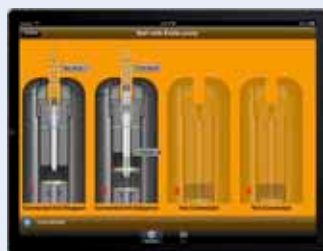
Fig. 310: iPad mini App for ExiGo pump showing sample volume to be dispensed from each pump
