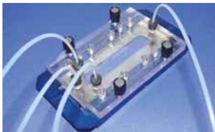
Fig. 177: Fully assembled MicCell with 25x75 Channel Plate, cross-shaped with 3 inlets and 1 outlet
