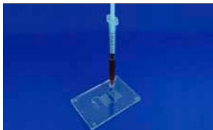
Fig. 466: Boyle-Mariotte PCR chip for ultrafast PCR, design: IMM, realized within the FP 7 project "CD-Medics", No. 216031
