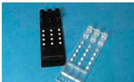
Fig. 162: IFSA 1 Immunoassay Chip – Equipped for three different samples with two measurement frits, one positive and one negative control frit
