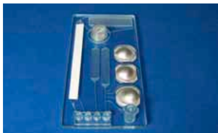
Fig. 232: DNA analysis chip with blister and integrated lateral flow strip
