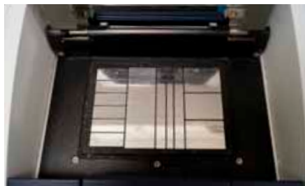
Fig. 267: Heating zones of ChipGenie® edition T2 and T2O
