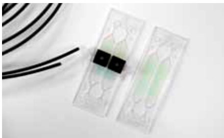
Fig. 481: Microfluidic chip with integrated oxygen sensing, FP7 project Biointense, No. 312148, responsible partner TU-Graz
