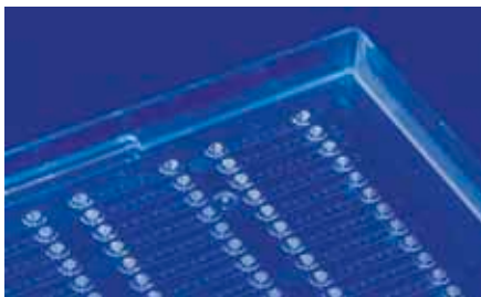
Fig. 26: Microfluidic titer plate with spotted probes
