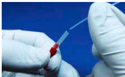
Fig. 247: PTFE tube connected via silicone sleeves to Mini Luer fluid connector
