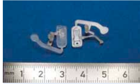
Fig. 453: Two component microinjection molding – Device for agglutination based assays, realized within the BMBF project FASAMOS, FKZ 02PC2001
