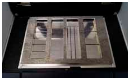
Fig. 268: Heating zones of ChipGenie® edition T2 and T2O with chips
