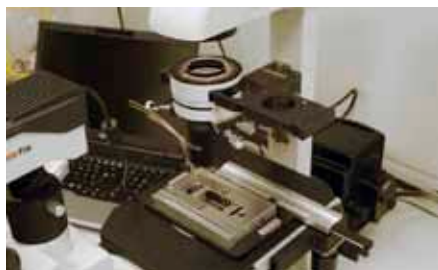
Fig. 298: Lab-on-a-Chip Cell Culture Incubator – LOC CCI 1 placed on a microscopy stage
