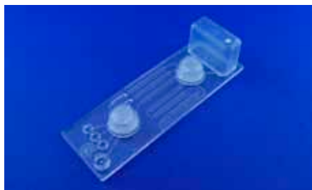
Fig. 467: Enzyme-assay development chip, realized within the FP 7 project Multisense Chip, No. 261810
