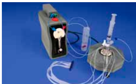
Fig. 312: Mirus Evo Nanopump with MultiFlow8; controlled by PC software, VenaFluxAssay (included)
