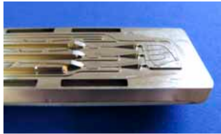
Fig. 411: Mold insert realised using ultraprecision mechanical machining
