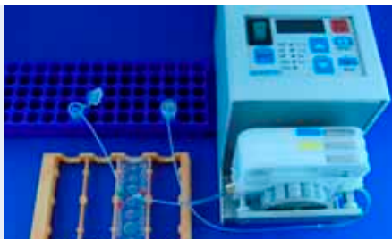
Fig. 368: Connection of pump via a PTFE tube with a liquid reservoir
