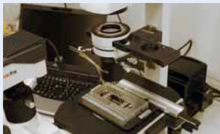
Fig 405: Lab-on-a-Chip Cell Culture Incubator – LOC CCI 1 during use on microscope stage
