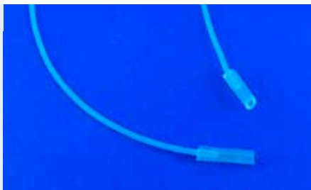
Fig. 382: Short pieces of silicone tubes connected with PTFE tube
