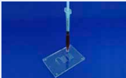
Fig. 369: Microfluidic chip with Luer interfaces filled with a standard syringe
