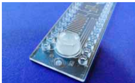
Fig. 461: Fluidic chip with rotary valve
