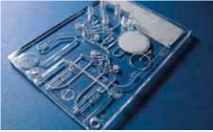
Fig. 452: Hybrid chip for immunoassays with plasma generation unit for electrochemical detection, realized within EU-FP6 project "SmartHEALTH", No. 016817
