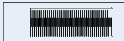
Fig. 275: Schematic drawing of 41-cycle continuous-flow PCR chip
