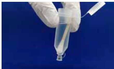
Fig. 241: Sampling vessel prefilled with buffer and inserted swab
