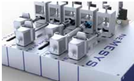
Fig. 304: Starter unit combined with different syringe pumps
