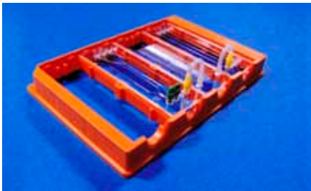
Fig. 62: Rhombic chamber chip in handling frame connected to PCR chip
