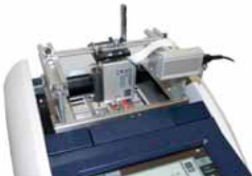
Fig. 346: Implementation of low-volume real-time PCR on chip – Chip on breadboard instrument
