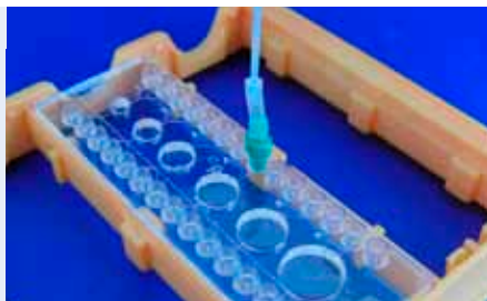
Fig. 364: Insertion of the Mini Luer with tubings in fluid entrance of the chip
