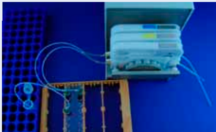
Fig. 378: Connection of the chip via the PTFE tube with the pump
