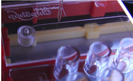
Fig. 185: DNA-array embedded in a microfluidic channel
