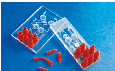
Fig. 116: Prototyped analytical platforms with Upchurch Nanoports
