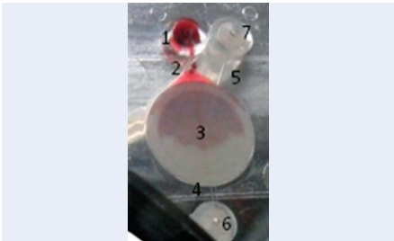
Fig. 80: Close-up of one plasma/serum generation unit
