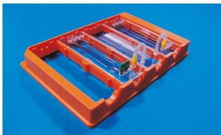
Fig. 50: Rhombic chamber chip in handling frame connected to PCR chip
