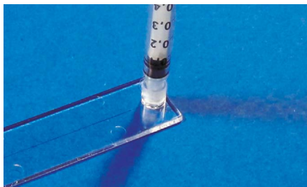
Fig. 32: Cross-shaped channel chip with female Luer interface and a syringe as male counterpart
