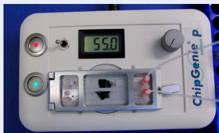
Fig. 193: Beads on chip during clean-up and elution
