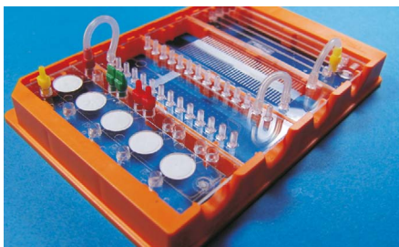
Fig. 137: Handling frame with different chip types connected with each other
