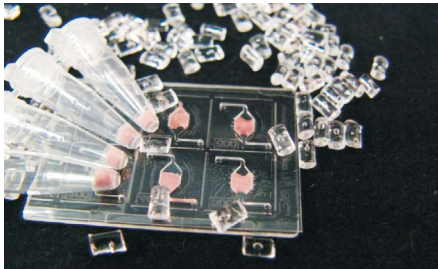
Fig. 234: PCR chip with integrated freeze-dried master mix
