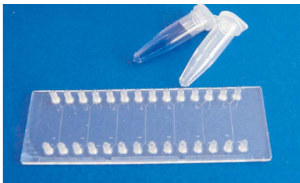
Fig. 209: Example of microscopy slide olive platform with 28 olive fittings
