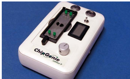
Fig. 160: ChipGenie® edition P instrument with bead-filled sample-prep chip
