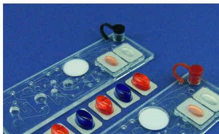
Fig. 251: Immunoassay chip with plasma generation unit and blister pouches
