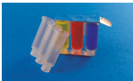
Fig. 120: Filled tanks sealed with alumina foil
