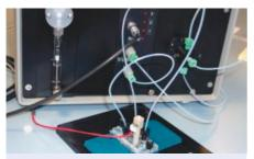
Fig. 113: MicCell FP-1-1-standard Fluid Processor. Foreground: MicCell with hydrogel valve in its blue support and black adapter plate
