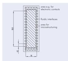
Fig. 116: Principle drawing of a microscopy slide with fluidic interfaces – in this version, fluidic interfaces are grouped along the long sides of the chip.
