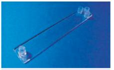
Fig. 31: Cross-shaped channel chip with Luer interfaces
