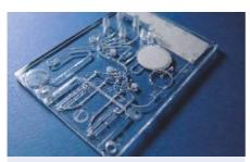
Fig. 156: Hybrid chip for immunoassays with plasma generation unit for electrochemical detection, realized within EU-FP6 project "SmartHEALTH", No. 016817
