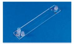
Fig. 38: Cross-shaped channel chip with electrodes for contactless conductivity detection
