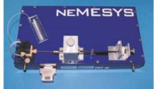
Fig. 112: cetoni neMESYS syringe pump system in use
