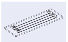
Fig. 13: Schematic drawing of the four-channel Mini Luer chip family
