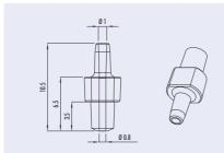
Fig. 69: Schematic drawing of a Mini Luer connector
