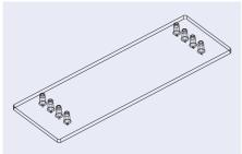
Fig. 122: Microscopy slide olive platform – version with eight fluidic interfaces
