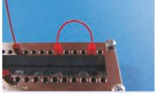
Fig. 86: Capillary PEEK tubing in use with nuts of the Upchurch Nanoport set in combination with a chip adapter frame
