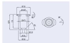
Fig. 75: Schematic drawing of the Luer Lok compatible adapter
