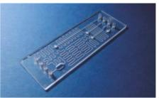
Fig. 159: Microfluidic chip for a complete SELEX-cycle, realized within the ETB project Artamis, FKZ 03139428
