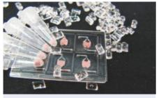
Fig. 150: PCR chip with integrated freez-dried master mix
