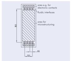
Fig. 117: Principle drawing of a microscopy slide with fluidic interfaces – in this version,fluidic interfaces are grouped along the short sides of the chip
