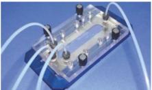
Fig. 63: Fully assembled MicCell with 25x75 Channel Plate, cross-shaped with 3 inlets and 1 outlet
