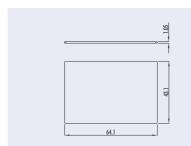
Fig. 140: Schematic drawing of 1/4 microtiter-plate
