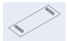
Fig. 130: Microscopy slide Mini Luer platform – version with eight fluidic interfaces  $\,$
