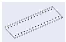
Fig. 120: Microscopy slide through-hole platform – version with 32 fluidic interfaces
