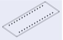
Fig. 119: Microscopy slide through-hole platform – version with 28 fluidic interfaces
