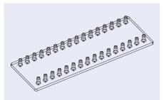
Fig. 124: Microscopy slide olive platform – version with 32 fluidic interfaces
