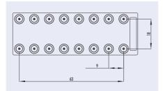
Fig. 126: Microscopy slide Luer platform – version 16 fluidic interfaces
