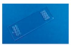
Fig. 133: Microscopy slide Mini Luer platform – version with 16 fluidic interfaces on the short edges
