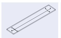
Fig. 33: Schematic drawing of the cross-shaped channel chip with electrodes
