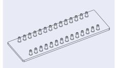
Fig. 123: Microscopy slide olive platform – version with 28 fluidic interfaces
