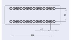
Fig. 134: Microscopy slide Mini Luer platform – version with 28 fluidic interfaces on the long edges
