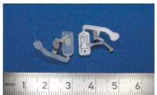
Fig. 157: Two component microinjection molding – Device for agglutionation based assays, realized within the BMBF project FASAMOS, FKZ 02PC2001
