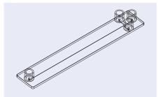
Fig. 29: Schematic drawing of the cross-shaped channel chip
