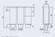
Fig. 82: Triple tank
