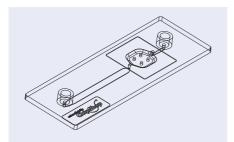
Fig. 23: Schematic drawing of a straight channel chip with additional large chamber
