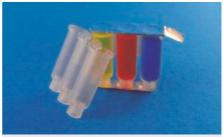
Fig. 80: Filled tanks sealed with alumina foil
