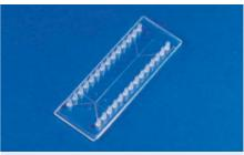
Fig. 149: Cell sorting chip
