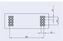
Fig. 132: Microscopy slide Mini Luer platform – version with 16 fluidic interfaces on the short edges
