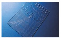
Fig. 158: Sample-in-result-out DNA-analysis chip, realized within the BMBF project ChipFlussPCR, FKZ 13N9556
