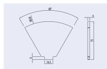
Fig. 146: Geometrical layout of the pie slice plate
