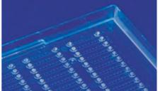
Fig. 22: Microfluidic titer plate with spotted probes
