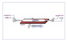
Fig. 107: Principle of a bead-based assay with the ChipGenie® edition P instrument
