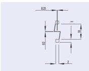
Fig. 105: Details of the electrodes
