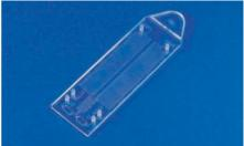
Fig. 153: Continuous-flow PCR chip, chip, realized within the BMBF-Project "ChipFlussPCR", FKZ 13N9556
