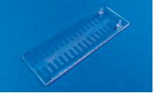
Fig. 96:15-cycle continuous-flow PCR-chip
