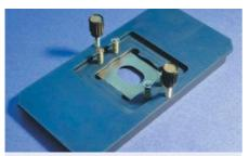
Fig. 60: MicCell support for 22x22 Channel Plates, to be placed in an inverted microscope via an adapter plate (not shown)
