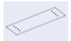
Fig. 118: Microscopy slide through-hole platform – version with eight fluidic interfaces
