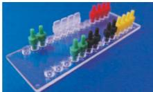
Fig. 135: Microscopy slide Mini Luer platform – version with 28 fluidic interfaces on the long edges
