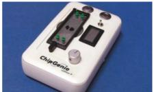
Fig. 108: ChipGenie® edition P instrument with bead-filled sample-prep chip
