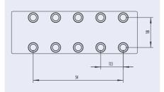
Fig. 128: Detail of the microscopy slide Luer platform with ten fluidic interfaces
