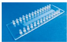
Fig. 98: 36-cycle continuous-flow PCR chip
