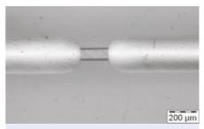
Fig. 106: Microscopy image of electrodes over microchannel
