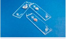
Fig. 83: Tanks mounted on a microfluidic chip
