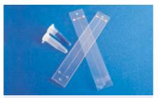
Fig. 36: Cross-shaped channel chips with through holes and electrodes
