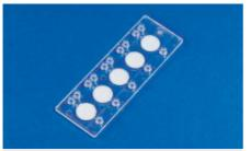
Fig. 152: Hybrid chip consisting of polymer and filters for plasma generation
