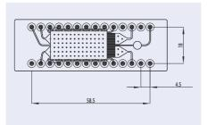
Fig. 47: Details of the field flow fractionation chip
