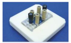
Fig. 66: Casting Station 22 mm x 22 mm. Top: assembled, including channel spacers (brown)
