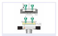
Fig. 57: Molding of the Channel Plate on a silicon master and subsequent mounting in an inverted microscope
