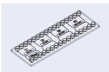
Fig. 39: H-shaped channel chip
