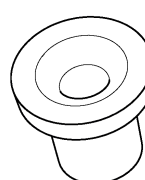
Schematic drawing of the male Luer plug Fluidic 270
