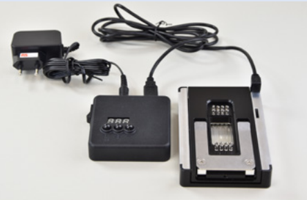
The complete setup of a LOC CCI 1 with heating elements. In contrast, the LOC HP does not include temperature control units.
